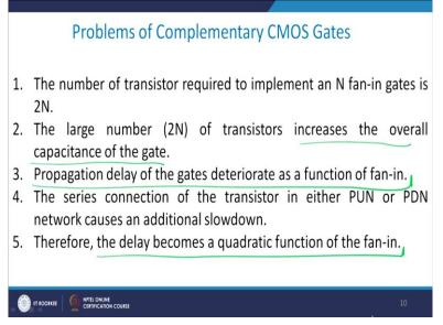
Let us look at the problems of complementary CMOS. Therefore the problem with complementary CMOS logic is that for N input, you require at least 2N Gates. That we have already seen. For example, two input NAND gate, I require two PMOS<sub>S</sub> and two NMOS<sub>S</sub>. For 3 input NAND gate, I will require three PMOS<sub>S</sub> and three NMOS<sub>S</sub>. So for an N input NAND gate, NOR gate, I require 2N number of gates and therefore the area is relatively large.
