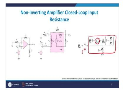
If I do a non-inverting exactly the same happens, non-inverting case  $R_{if}$  case comes out to be equal to this one right and this is sorry this is actually  $V_I$  by  $I_I$ , right, input current and this is the input resistance 1 plus  $A_{OL}$  plus  $R_2$ .
