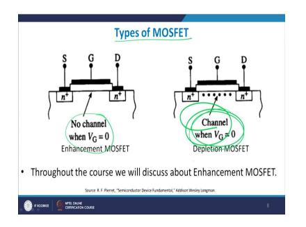
No channel when  $V_G$  equals to 0 for enhancement mode MOSFET. For depletion mode MOSFET, when  $V_G$  equals to 0, you still have some channel being formed here right? And that is quite an interesting phenomena as far as types of MOSFETs are concerned.
