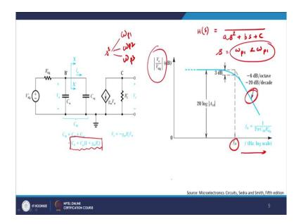
And with this if you plot again, exactly the same thing as your previous case, so common source and common source MOS amplifier and common emitter bipolar transistor, high-frequency looks almost the same, qualitatively as well as most quantitatively. So, if you plot again, therefore gain versus frequency and you see that your cut-off frequency  $F_H$  comes out of the again somewhere here, which depends upon the value of  $C_{in}$  an  $R_{Sig}$ ', right.
