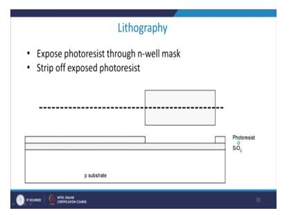
So, let me come to lithography, you need to expose the photoresist through an n-well mask, right? And then a sign of strip off the photoresist. Once you do that you are stripping off your all other things. So, what you do is that this is basically you're the photoresist that has fallen on to this bank this bank. And as a result, you strip off the photoresist from this directly, right?
