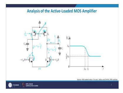
2 and 4 is basically  $C_{GS2}$  and  $C_{GS4}$ .  $C_{gs2}$  is gate to source of gate to source of 2 plus gate to source of 4,  $C_{GS4}$ . These 2 will be again parallel.
