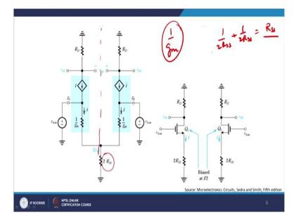
Therefore, as I discussed with you just now and I was deriving also with you. Do a half circuit here, remember? I remove the MOS device here and show it as a current source in series with 1 by  $g_m$ , remember because looking at the source side the amount of resistance offered is actually equals to 1 by  $g_m$ .
