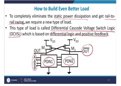
So let me see how can you build a better load or maybe a good one. And this is known as what is known as a Differential Cascoded Voltage Switch Logic, DCVSL. Differential Cascoded Voltage Switch Logic, also known as DCVSL, based on differential logic and positive feedback. So what you do is very simple. You have a PDN and you took a PDN2 which is just complementary of PDN1 and you apply both A and its, so if you have two signals, you also apply its complementary signal and what it does?
