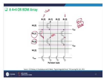
Let us look at the 4 by 4 ROM array. In this ROM array it is all MOS based ROM array and therefore let us suppose your WL[1] is high then what it does is, this  $V_{DD}$  through these appears on bit line, so your bit line equals to  $V_{DD}$ . Similarly if your WL[2] is high then I ensure that  $V_{DD}$  is written onto BL[1], similarly if WL[2] is high then I will ensure that this  $V_{DD2}$  is written on this bit line
