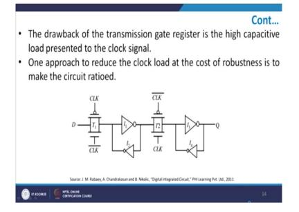
Now the drawback of transmission gate register is the high capacitive load, we all know this point, because you remember this transmission gate obviously terminates with both PMOS and NMOS on the same substrate and therefore you will have excessive loading of the substrate onto the device itself and as a result you will have large amount of capacitive delay.
