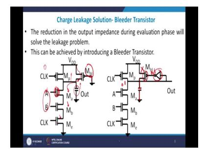
So, what people thought and people did also, they introduced what is known as a bleeder transistor. Now, let us see how it works out very simple and straight forward. What I do is I have  $M_a M_b$  so it is an AND gate. This is my evaluation transistor here and this is  $M_a$  input 1 input 2 A and B are inputs here CLK and I have put a bleeder transistor  $M_{b1}$  there right? So let us see how it works out. So let me say that CLK is basically equals to 0.
