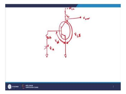
So let me just draw for you from the circuit point of view, right and let us see a common emitter configuration works in a sense in this case. So I have an RC here I have a base resistance  $R_B$  here and since this is NPN so I can just do like this, right and we can vary this one to a larger extent and maybe I can reverse maybe I can fix the value of voltage +V<sub>CC</sub> here. And we will try to take the value of V<sub>out</sub> from this place particular place, right.
