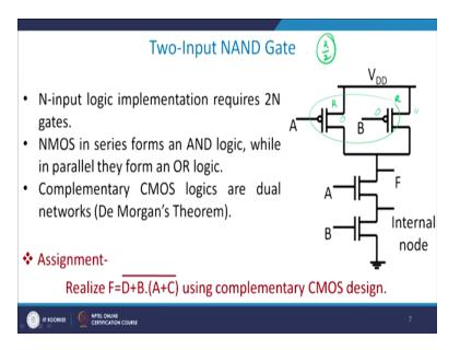
These two  $PMOS_S$  are in parallel which means that if both are 0, both are on and therefore if each carries a resistance of R, then the actual resistance is actually equals to R/2. So the resistance between F and  $V_{DD}$  rather than being R is now R/2 which means that I can pull up the voltage here to  $V_{DD}$  in a much easier manner. Agreed? So with this statement or with this knowledge, see what happens.
