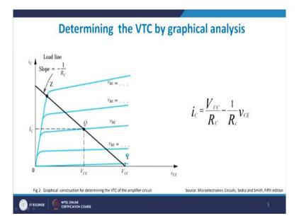
We now therefore come to determining the VTC by graphical method, right? How will you find out the voltage transfer characteristics graphically or looking at a picture at a graphical point of view, right? And that is what is required and I will discuss that in this section in this lecture, right? Let us take one important point, let us take BJT switch or the BJT transistor as an amplifier, right?
