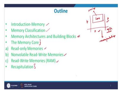
So the core will be actually storing the data and the peripherals will be responsible for manipulating the data which means that should be able to read or write the data. So primarily read and write will be responsible for the peripherals, so we are looking into that. Then we will look into ROM read-only memory and nonvolatile read-write memories and then readwrite memory as well and then recapitulate the whole thing and that is what the whole structure is all about.
