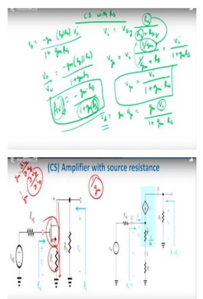
So this is a source degeneration resistance, which you see and I told you what is that advantage of source degeneration resistance, right. Let me therefore show you source degeneration, so CS stage with  $R_s$ ; let me just do some small derivation here, CS
