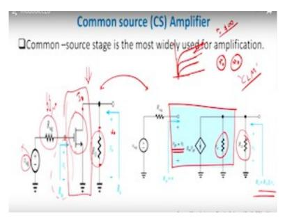
Common source amplifier is this, this is the diagram of a common source amplifier, right. This is the diagram of a common source. You see here you have a NMOS device which is this one active device, this is your output resistance of the input signals source, so this is the signal source which is there with me, right.
