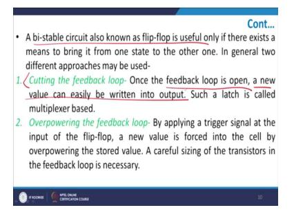
Now with this knowledge a bi-stable circuit can also be known as flip-flop, why flip-flop? Because they are two stable states and by doing some manipulation I can move the stable state from A to B and I can also bring it back from B to A right. I will show to you how this is done. There are two basic approaches by which you can achieve a bi-stable circuitry, obviously you should cut your feedback loop and therefore now the feedback loop is open and now you can write very well onto the output.
