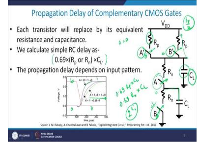
Now what we do is that, we replace each transistor by a switch and a resistance. So whenever my device is in the on state, this will, whenever my A equals to 0, this will go down. So therefore I write A complement and B complement. When I say A complement and B complement, I mean to say 0 means the switch is on and 1 means the switch is off. Whereas for A and B, when A is equals to 1, it switches on. A equals to 0, it switches off.
