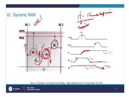
Now another example is basically my DRAM which is dynamic RAM and it is consisting of also referred to as 1T-1C design which is one transistor, so this is one transistor and one capacitor and therefore if you see very closely even WWL is high, which you see, this is high. This high means  $M_1$  is switched on, when  $M_1$  switches on The bit line is suppose 1.
