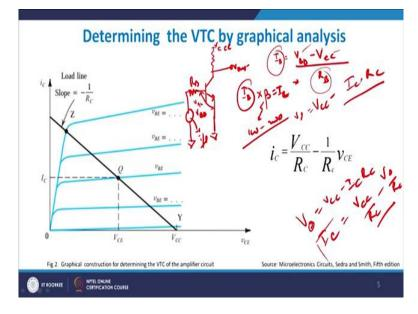
So what was the concept is that in a common emitter mode configuration, let me draw for you the common emitter mode configuration design, right? And this is without the collector emitter configuration  $V_{cc}$ , right? You had  $R_B$  and then you had  $V_{BB}$  and then you had this and then on the emitter side you had this, this is your output and this is your input which is basically a sinusoidal input.
