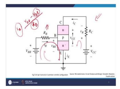
If you look at  $V_{BB}$  this is my  $V_{BB}$  and this is my  $R_B$  right. So I get  $I_B$  to be equals to  $V_{BB}$ , right, if you go from this side to this side  $V_{BB}$  -  $V_{BE}$  right base to emitter junction divided by  $R_B$ . This is 0.7 this has to be of the order of few kilo-ohms for this to be in the order to few
