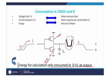
Then let us see what happens when your input goes from zero to 1, so I have initially zero and then it goes to 1, so initially zero means this is ON state this is ON right, and this is OFF, right and therefore, this whole  $C_L$  is filled with water which means that this  $C_L$  is actually 1, voltage across the  $C_L$  is actually equal to  $V_{DD}$  and now I go from zero to 1 which primarily means that this goes from ON to OFF state and this OFF it goes to OFF to ON state.
