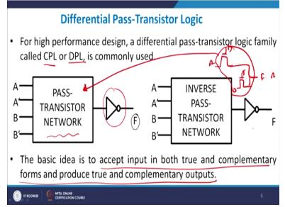
Now, typically when you do a high-performance design, we use a differential pass transistor logic in which we assume that my input and its complements are available to me. So A, A bar, B, B bar, C, C bar, are all available to me and I do a pass transistor network here and then I put a static inverter to get a full swing in the output side.
