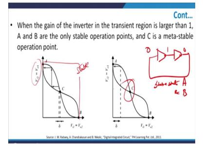
You will have a stable state at A, so stable states are what? Stable states are A and B, any other state is sort of an unstable state, the most unstable state is basically the C where you have got two VTCs crossing each other, why crossing? Because input of two is exactly goes to the output of one. So I am just overwriting each one over other and I get this into consideration, A and B are the most....
