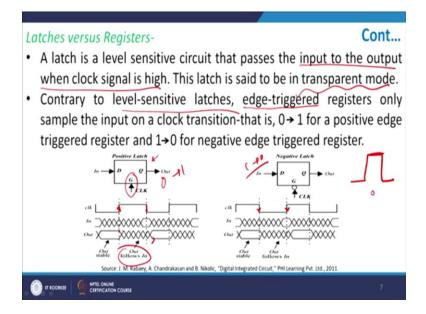
So with this knowledge let me explain to you the difference between latch and register, you must be knowing also, latch is a level sensitive circuit and passes the inputs to the output when the clock signal is high. So this is my latch, so whenever at this state when the it is level, when it is level sensitive and high level it is reached, then only the latch becomes transparent and is able to perform any operation and let the input go to the output with the clock is high.
