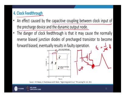
Last, let me come to the last problem area of this thing and this is what is known as a clock feed through. Clock feedthrough is basically a capacitive coupling between the clock input of the precharge device and the dynamic output node. So if you look back here this was clock here and this was the output here. So your clock goes high like this right? Now because of a coupling between this and this, the node voltage also goes like this.
