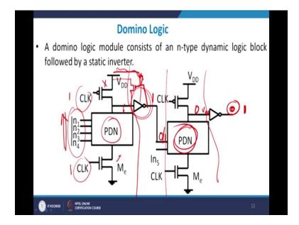
How you can do that sorry how you can do that, you can add a bleeder transistor here right and this bleeder transistor will be added here and this will be  $V_{DD}$  it will be taken care of in this manner and therefore you can have a bleeder transistor directly inserted here. So charge loss will be taken care of. The charge sharing will be taken care of and the domino logic gives you a very good idea about this whole charge description.
