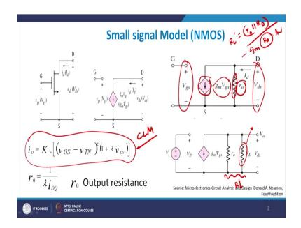
So, I just take  $r_0$ , in parallel to the current source here, where,  $r_0$  is basically, the resistance offered by the device, when the device is operating in the saturation region, fine. And therefore, there will be a current I<sub>d</sub> flowing here, there will be V<sub>ds</sub> flowing here, and this  $g_m V_{gs}$  is current.
