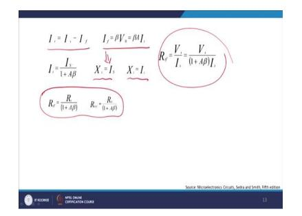
Now, therefore I get Ii the input current equals to  $I_s$ - $I_f$  because of negative feedback. We already if to be equals to  $\beta * V_0$  and this is  $V_0$  is nothing but  $A*I_i$ . I can safely write down if to be equals to  $\beta * A*I_i$ , right? So, I get  $I_i$  equal to therefore equals to  $I_s / (1+A\beta)$  and therefore I can safely write down input impedance or input source is basically  $X_s$ .
