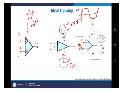
The reason is see I discussed with you just now that in the previous slide that this is limited by plus  $V_{CC}$  and minus  $V_{CC}$ . So if your plus  $V_{CC}$  is plus 15 and let us suppose this is minus 15 volts right. You do anything you want to do, the  $V_{out}$  value cannot exceed plus 15 in the positive cycle and cannot exceed minus 15 in the negative cycle because these are limited by the power supply here. And if it crosses there will be clipping.
