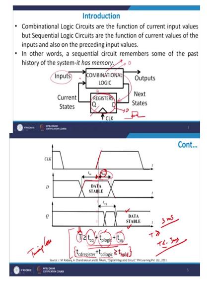
The combinational logical block here, this delay plus this delay, right plus the setup time here is defined as my combinational logic as the total, as means....it is basically your stability criteria and the minimum time should be actually the sum of all these 3. That means if you say, say this is 1, 1, 1, so let us suppose 3 millisecond. If t is greater than equal to 3 millisecond, no issues, if t is less than or equal to 3 millisecond then there is a problem.
