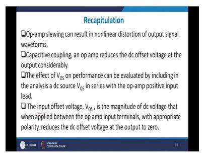
So let me recapitulate what we did, we were actually looking into an op-amp slewing action. What is the meaning of slew right and what is slew rate, slew rate limited operation? What is a DC offset voltage right and how do you define DC offset voltages? What is the meaning of saturation, operational amplifier saturation? What is the meaning of input offset voltage Vos?
