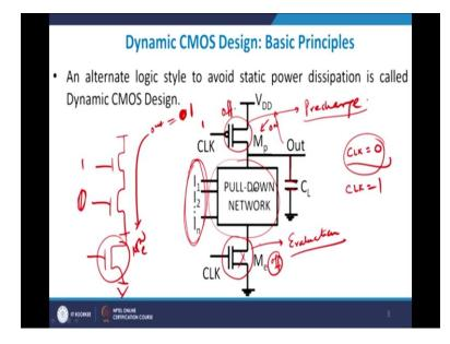
Now let us come back to dynamic logic and see how it is removed. Dynamic logic you have one single pull-up just like your CD NMOS inverter PMOS and you also have an evaluation transistor known as  $M_e$  and so this is an NMOS also referred to as an evaluation transistor  $M_e$  and this is  $M_p$  also known as a pre-charge transistor. We will explain these terms individually but we will come to that later on.
