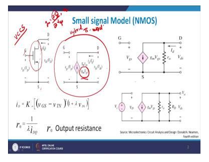
Now, let me come to you, the small signal model of the FET device. If you look here carefully, this is the N-MOSFET, which is in front of you, right. I have a current flowing which is a drain current.  $V_{ds}$ , is the drain to source voltage, which you see here. And you have a gate to source voltage, which is available at this particular point. So, it is basically a three terminal device gate, drain and source.
