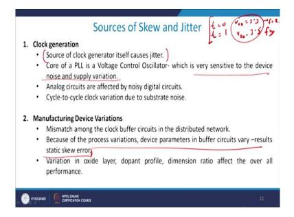
Now the source of clock generator itself causes the Jitter for example generally we use VCO which is voltage control oscillator or even PLL which is responsible for generating the clock but the problem is these are very very sensitive devices and they are prone to noise and supply variation. So even if your  $V_{DD}$  which you have supplied is changing by even a fraction of amount that frequency will change slightly and therefore that gives you a Jitter.
