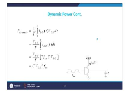
As I discussed with you dynamic powering, I will not go into further details of it, but I will give you a brief idea about dynamic power dissipation, it is actually  $V_{DD}$  by T f SW t times f SW is basically the frequency operation or number of times the output change before time t and this is what is known as this thing. We came to dynamic power dissipation given by  $CV_{DD}$  square times f of SW, f of SW is the frequency of your short way, the frequency of your wave.
