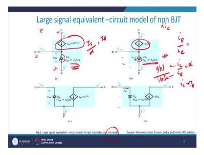
Now onto the emitter side this is the base and this is the collector on the emitter side we have a reverse biased PN junction why we have already seen this why. The reason being that at this stage since emitter base junction when you are using in an active mode because we are using this in the active mode emitter base junction will always be reversed biased, right because it will be reverse biasing the emitter base junction.
