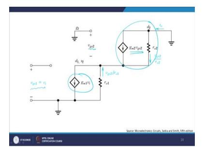
If you look very carefully therefore, this is your cascode amplifier which is given by  $g_{m2} V_{gs2}$  is the current source and  $g_{m1} V_i$  is the q1 which you see and  $r_{01}$  and  $r_{02}$  are respectively the drain to source resistances offered by these devices. And as you can see here,  $V_{GS1}$  is nothing but  $V_i$  and  $V_{GS2}$  is nothing but shorting it. So, basically  $V_{GS2}$  is that which you see in front of you. I am shorting it, right?
