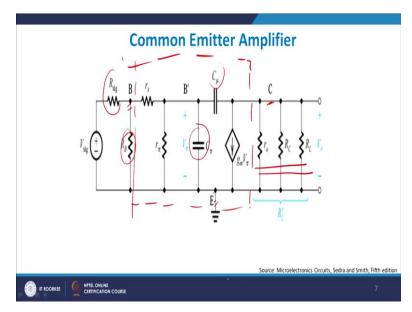
For the case of common emitter mode configuration let me come to common emitter amplifier, we have a BJ T based common emitter amplifier. So, now you have, this is the base, right, this is the collector and this is the emitter. Now, this is your signal, so this is your signal and this is your base resistance which you see, right,  $R_B$ . So  $R_G$  there is analogous to  $R_B$  here and  $R_0$ ,  $R_C$  and  $R_L$  are effective load in the output side.
