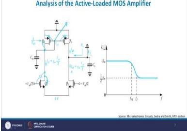
Let me show to you therefore id. So, total current which is flowing through the device is nothing but  $i_{d4}$  plus  $i_{d2}$ . What is  $i_{d4}$  and  $i_{d2}$ ?  $I_{d4}$  and  $i_{d2}$  is nothing but this is  $i_{d4}$  this is  $i_{d2}$  and this is  $i_{d4}$ . So, if you look at  $i_{d4}$ , this is the total current which flows through a device. This can also be written as gm into V<sub>ID</sub> by 2, right because that is the current which is flowing through the arm.
