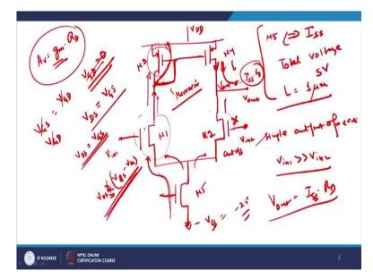
It is not grounded here but this is VDD which is plus 2.5 and we have got minus VSS which is basically minus 2.5 and therefore the total swing, the total voltage available, swing available to me is basically equals to 5 volts, right? And this is L equals to 1 micron
