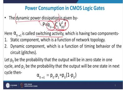
With this knowledge, what we do is we define another term known as dynamic power dissipation. It primarily means that, whenever the inverter is in operation mode, operation in the sense that whenever your input is varying from 0 to 1 and 1 to 0 and there is a large input bit train coming into picture and the output is also therefore varying from 0 to 1 and 1 to 0 we define this to be as a dynamic operation. What is a static operation? Static means that when it is given 1
