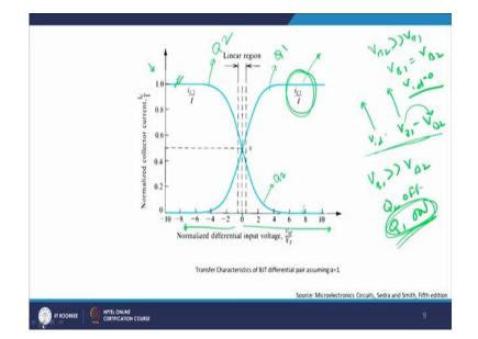
Now, with this knowledge which you have gained till now, right let me just therefore give you a small idea about the transfer characteristics. Now, on the y axis you will see it is basically the normalized collector current which means that collector current normalized with respect to the total current which is available to us and therefore the maximum I Can go is 1 and on the x axis we have V <sub>id</sub> by  $V_T$ , V <sub>id</sub> is basically the difference voltage of the base
