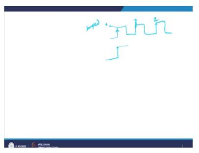
Suppose let us suppose I have a clock here and whenever my clock goes high, my data which is coming from outside gets inserted into the system. So, I will get here data will be inserted, here data will be inserted and here data will be inserted or in technical terms these are referred to as the data will be sampled at these particular points, at x, at y and at z. And so
