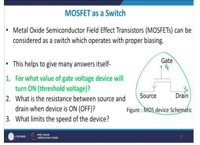
So you see this drain, you will apply a potential here, here you apply a potential  $V_D$ , here you apply a signal or a potential  $V_G$  and generally source is grounded right. So 1, 2, 3 that will, we are not looking at substrate nowadays at this point. But we will see how it works out.
