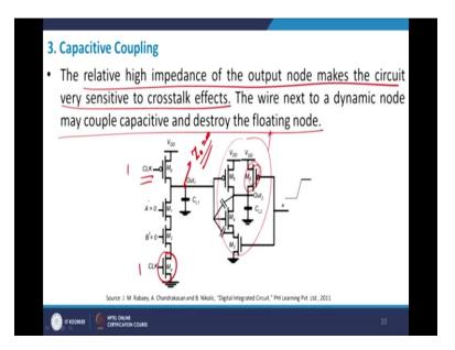
Let me discuss with you the capacitive coupling therefore. The capacitive coupling, so my output impedance is relatively high and therefore very sensitive to cross talk effects. That is the only problem area of a dynamic logic because this is quiet high  $Z_{out}$  is equals to infinity ideally right? The wire next to the dynamic node may couple capacitive and destroy the floating node right and that is your problem area which you face for a dynamic logic design.
