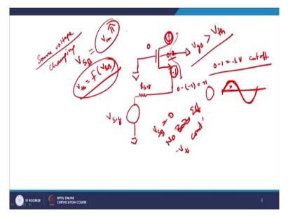
One small problem area of Common Gate. So, please understand, you are feeding the signal from this  $R_{sig}$  right,  $V_{sig}$  right and this is  $R_{sig}$  and you are feeding on to the source terminal of the battery. And the gate is grounded, right. If you look very carefully, when this, so for the device to be on, gate to source voltage should be larger than the threshold voltage of the device. That is the basic concept we have been learning for, we know very well.
