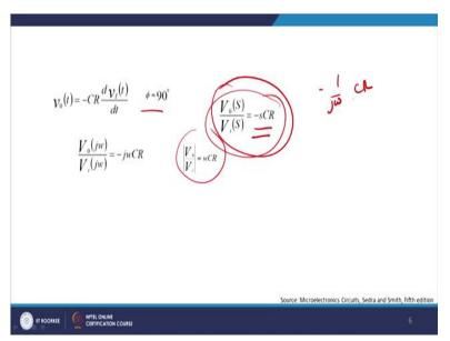
Exactly, the same thing as I did it in the previous turn,  $\phi$  equals to 90 degree, I get output voltage V<sub>0</sub> by V<sub>R</sub> equals to minus s times CR, right. So, minus S is minus 1 by j $\omega$  into C into R, right and that what gives you the value of your output voltage.
