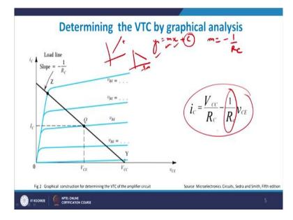
Which means that if you look very carefully or even if you look at this particular point I can safely say that this is the final content that the collector current is only depending on the value of  $V_{cc}$  by  $R_C$  and it depends upon minus 1 by  $R_C V_C$  which means that if you compare with the fact Y equals to  $m_x$  plus c, m is basically your 1 by  $R_C$ , right? So why with the negative sign because the slope is negative, right?
