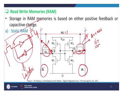
Let us look at the static RAM and one of the first example of a static RAM is basically your 6T cell or 6 transistor cell. So if you look very carefully this  $M_5$  and  $M_6$  are referred to as access transistors and this is basically cross coupled inverter so if you just do one small job here it looks something like this, it looks something like this. So this is your word line and this is your bit line and bit line bar. So this is your bit line bar and this is your bit line.
