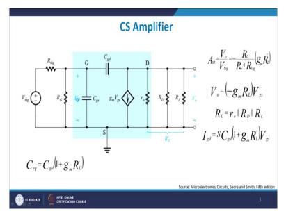
This is the small signal diagram for common source amplifier.
