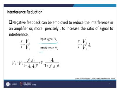
So, I will just show you what I am trying to tell you here that I have an input signal which is Vs, I have an interference which is  $V_n$ , so this is my noise voltage, input referred noise voltage. So I have Vs by  $V_N$  which I get and therefore I signal by interference S by I is Vs by  $V_n$  into A<sub>2</sub> because A<sub>2</sub> is nothing but this signal where am getting it.
