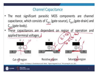
Now let us come to the channel capacitances, now channel capacitance as I told to you will have again two components primarily. We have understood  $C_{GS}$ , so it is basically gate to source, so it is gate to sorry, this is  $C_G$  gate, channel source, you have gate drain, so gate drain and then gate body, so this is gate to channel, this is gate to channel and this is also gate to channel for three regions of operation for cut-off, for resistive region and for saturation region right.
