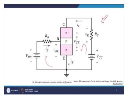
I will make it a much better diagram from the point of view of understanding which is this one, right. So I have an NPN transistor, I have a BJT and I have my base emitter junction forward biased, right and my collector base junction to be as reverse biased this one right. (Refer Time Slide: 1:37)
