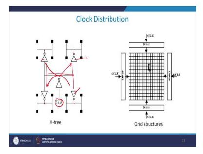
H-tree, I may have a diagram, yes. This is the H-tree which you see, so I have generated a clock here and using an inverter I generate the clock and then this is H. so this is your H and therefore this distance, from this point to this point, this point to this point, this to this and this to this are exactly same. Assuming that the delay of these inverters are exactly the same.
