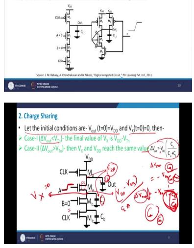
The classic problem of this thing is that when you have a capacitive coupling between the two we also have a charge sharing. What does a charge sharing mean? Charge sharing means that whenever your device switches off, the charge which is there within the device has to sit somewhere right? It has to go somewhere right? And therefore, it will, that charge will be shared between two or three devices and its voltage will go up.
