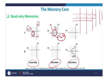
And therefore for example if the word line is high these diode switches on and one appears on the bit line a very straightforward and simple. Similarly when the word line height this MOSFET switches on, this  $V_{DD}$  appears here at a particular point of course there will be one threshold voltage drop of the transistor but that is immaterial at the stage. Similarly, so this is a diode based ROM.
