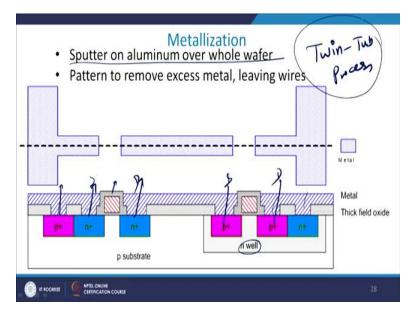
Once, you have grown the contacts which is this one; we have grown the contacts, we then sputter after we have grown the thick oxide layer. Now, my now my region where you want to grow the oxide is opened. Then what I do? I sputter with aluminium over the whole wafer. So, I do a sputtering using a sputtering technique; I sputter over a whole aluminium. The aluminium actually sits at those places which was opened, right?
