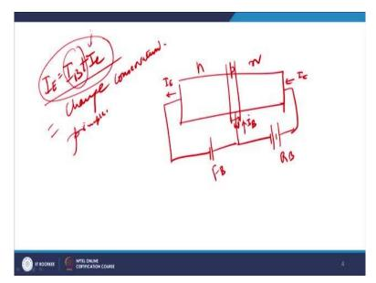
So if you look at very carefully  $I_E$  is equal to  $I_B$  plus  $I_C$  and therefore total emitter current in the system is sum of base current and collector current, right. And that is how you manipulate. So you try to therefore maybe control the flow of the collector current by increasing or decreasing the value of the base current right by changing the value of base current you can actually make  $I_C$  or  $I_E$  almost close to each other.
