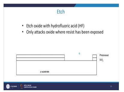
What is etching? Etching means that, You etch the oxide with Hf. So, I have an oxide formation means I want to remove it for whatever reasons. Then what I do is I put Hf or hydrofluoric acid
