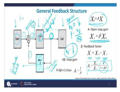
If you look very carefully it comprises of, of course source is there, right? Which will be responsible for giving a voltage or current and there will be of course a load. So for any electronic system you will always have a source and a load. The load might be a resistive load, a capacitive load but primary a load will be there across which you will be able to find out the voltage or current.
