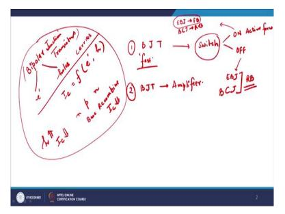
And these two things, the first thing is that BJT can be used as a, of course as a switch, right? So we can go from ON to OFF state, right? How can we go from ON to OFF state? This is
