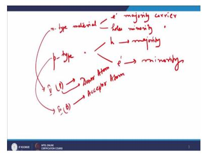
So and therefore let us comeback to an original issue to statement therefore that I have a n type material, I have a p type material, n type will have electrons as very large quantity and therefore electrons will be referred to as. So what we will say is in an n type material, I will be discussing or I will be knowing that electrons will be referred to as a majority carriers a majority carrier right and holes we will see why, holes will be referred to as minority carriers.
