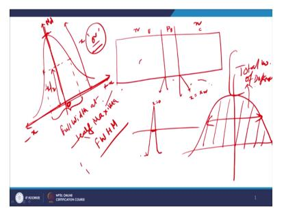
It is known as inverted dumbbell shaped doping profile. The idea here is this is known as this is maximum, right? And this is say, this is X. Then, this is approximately X/2 and we define this width, right? We define this width as full width at half maxima. Right?
