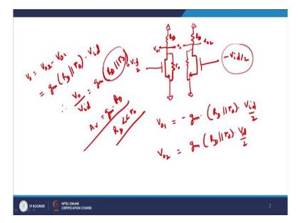
And let me show you how this works out. If I have got to circuits here, right? And they are primarily given like this and this is plus  $V_{id}$  by 2, this is  $R_D$  and then this is again the same here. So there are 2 half circuits which is here and then this is the series resistance of the device itself, so this is Ro, this is  $R_D$  and this is again V0 output voltage which we are trying to find out and this is minus  $V_{id}$  by 2.
