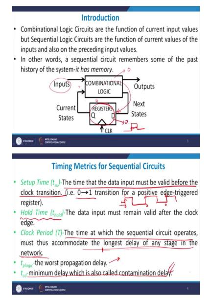
C to D is basically referred to, if you back the previous slide, C to D is basically this to this delay, right, overall delay. This has to be actually very small or it should be very small. Contamination delay should be 1. So if you want the sequential logic to move fast, you need to reduce these delays drastically.
