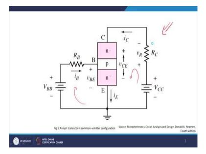
This is the active common emitter mode configuration active source forward active mode configuration with the schematic shown in this figure.
