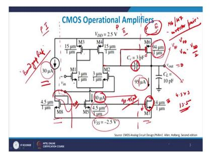
Now that is the general scheme of things which you see now. You do have a capacitor here which is basically a role of a blocking capacitor because it does not let any DC component to pass through it and reach to this particular point it only reads the A/C component to pass through it because you don't want any DC component to load your subsequent stage. The subsequent stage now is basically your P3, right?
