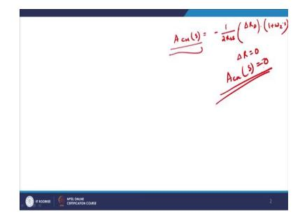
So, RSS is relatively very high and as a result what you will see is  $A_{CM}$  is very low in that case. So, when I go in frequency domain I replace  $R_{SS}$  by  $Z_{SS}$  and  $Z_{SS}$  is given by RSS parallel to  $C_{SS}$ , right? And we get  $R_D$  upon this thing into consideration. Now, 1 upon  $Z_{SS}$  is nothing but  $Y_{SS}$  and therefore, I get  $A_{CM}$  to be equals to minus  $R_D$  by 2 into del  $R_D$  by  $R_D$  into  $Y_{SS}$ , right?
