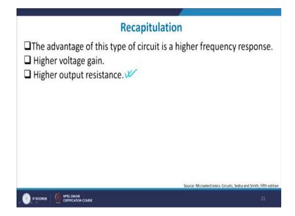
So, let me recapitulate what we did in this in this case? We saw that if I do a cascoded amplifier in place of a differential amplifier, the gain will be relatively high at the cost of voltage head rooms; my gain will be also very high, right? That is what we have seen here. So, that is what you see here that they have got higher output impedances and they have got a higher voltage gain. So, cascoded transistor means CS and CG in series with respect to each other we define them.
