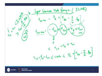
Plus you require  $V_t$  threshold voltage of the Q1 transistor and  $V_{overdrive}$ . You understand why these 2 are kept because otherwise the system will not get on. So your minimum common mode voltage should be this much that it should be able to switch on your device, draw the device into the active region by  $V_{overlap}$  and should sustain a minimum value of voltage between the source and through the current source otherwise it will not work fine.
