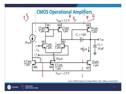
And therefore if you see its aspect ratio is very large, you see 4.5 by 1 micron. So this is design is based on 1 micron technology which means that channel length of all the transistors used here is approximately 1 micron. And the ratio if you look at W by L ratios of M5 is typically very high, right? It is 4.5 micrometer by one micrometer, right? And your VSS is latched to minus 2.5 volts, so it is not grounded here, if you go back.
