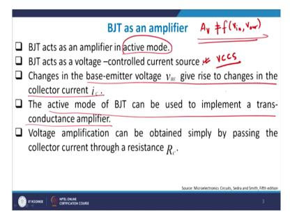
And therefore what we have learned just now therefore is that a change in the base emitter voltage which is this one gives rise to a change in the collector current  $i_c$ . I think this has been already discussed to a larger extent so for example if you are using a silicon transistor and your  $V_{BE}$  is less than 0.7 you can be amply sure that the emitter base junction is cut-off and therefore there is no current appreciable amount of current flowing through the emitter base junction.
