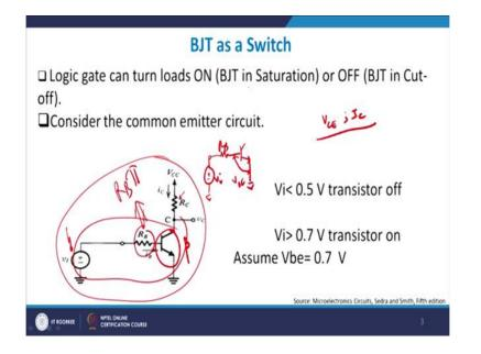
Because this is the, so I am concentrating at this place, right. So it is something like this now that I have  $R_B$ , right and then this, right and then, you have got  $V_I$ . So  $V_I$  minus  $V_{BE}$ , right, divided by  $R_B$  is your  $I_B$ .
