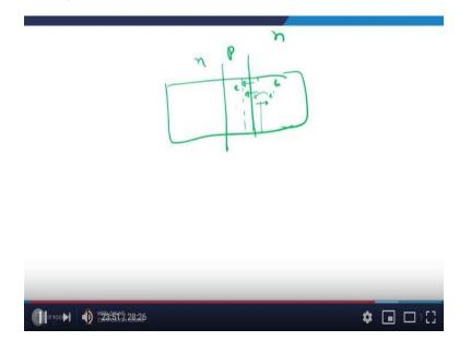
Now this...Once they start moving, so I have this junction, this is emitter based junction and I have got NPN and electrons are available here and holes are available here, right? So the electric field internally which is there in the depletion region between P and N because it is reversed bias so I have a depletion region here, right? (And I would expect) so the internal electric field will be from this side to this side.
