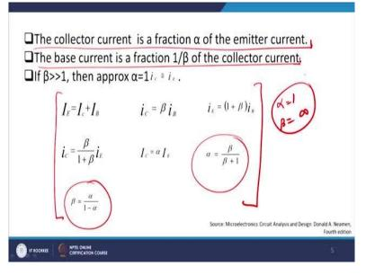
Right and then I was discussing the collector current is therefore is a fraction  $\alpha$  of the emitter current. And for  $\alpha$  is very close to 1 so if emitter current is 1 millamp you will expect to see collector current very close to 1 millamp because  $\alpha$  is very close to 1, right. And the base current is 1 by  $\beta$  of the collector current. This we have already seen just now in this case and these are the few important parameters found in the book also.
