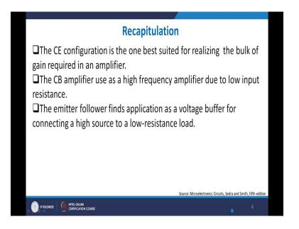
So let me recapitulate what we did. Common emitter configuration is the most easiest and the most high gain, can be obtained from common emitter configuration. The common base amplifier user high frequency amplified it with low input signal, right? Input signal is quite low and therefore you use a high amplifier design. The emitter follower finds application as a voltage buffer right, for connecting high source and passes it onto right source.
