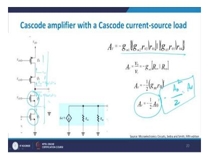
If you look at the cascoded current source which is being basically a current source which you see. So, this this is my input device q1 this is my cascoded device and these q3 and q4 are basically my load, right? And these loads will give you a value of voltage gain which is equals to  $a_0$  square by 2. This will be with a minus sign and you will get  $A_v$ , right?
