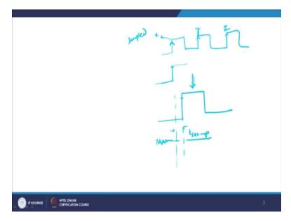
So, what I am trying to say is that, let us suppose my clock is rising here at this instance of time, right. So your data must be held stable, so your data is moving like this let us suppose, up and down, but minimum it should become stable at this particular point.
