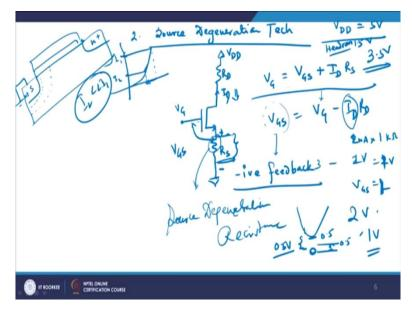
The second one which people follow is defined as source degeneration technique. This is source degeneration technique of biasing, so what I am trying do, I am trying to bias it from an external source using a DC bias, I am doing it on external source and trying to find out. Let me draw for you how it is different.
