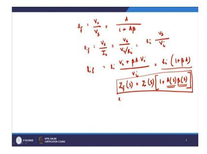
And let me write down therefore that with feedback I get  $V_0/V_s$  and that is equals to A/(1+ A  $\beta$ ) and that is a standard form of you see but let me write down, let me show a derivation of good impedance with feedback I get  $V_s/I_i$  output, source by current, I get  $V_s/(V_i/R_i)$  because  $I_i$  is the input current, which is nothing but the voltage, input voltage by input current and this can be written as resistance times  $V_s/V_i$  right.
