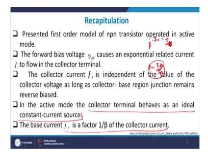
So let me recapitulate what we have learned till now, we have presented a first order equivalent NPN model operated in the active mode. Active mode is when emitter base junction is forward biased and collector base junction is reverse biased. Any forward bias profile or entity will always cause an exponential change in the value of current and therefore the collector current  $I_C$  is independent of the value of the collector voltage as long as the collector base junction remains reversed bias.
