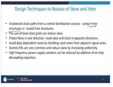
Okay how to reduce the Skew and Jitter. The best option available to you is try to make the clock as symmetric as possible and one of the example is basically H-tree.
