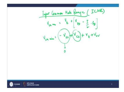
Now, what is the meaning of  $V_{CM min}$ , minimum CM voltage is minus  $V_{SS}$  plus  $V_{CS}$  plus  $V_t$  plus  $V_{overlap}$ . Now, obviously this could be grounded also, so this can be put to 0 otherwise it is connected to a negative terminal.  $V_{CS}$  is this voltage which I will just show it to you.
