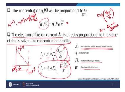
And let us see if we proceed forward it gives me an exponentially falling down, which means that though it is basically shown as exponential we approximate it as a linear fall concentration of electron as you can see. Therefore, if my  $V_{BE}$  would have been larger this is where the basic fundamental principles comes if
