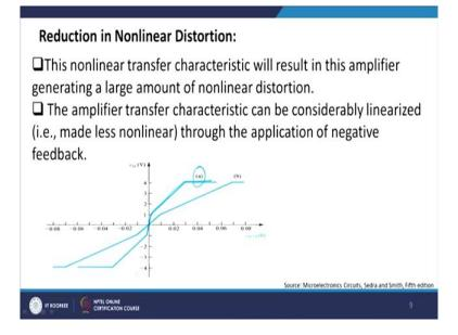
So when you do a negative feedback your non-linear distortions get reduced drastically, right? This is feedback and this is without feedback. With feedback it is almost linear in dimensions and nature whereas here you will have peace wise linear approximation because of, so when you apply a negative feedback distortion also reduces, right? The non-linear distortion also reduces drastically.
