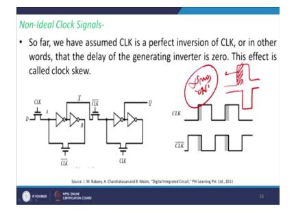
This is how you generate a non-ideal clock signal right. However there will be some delay between two clocks right and that is known as Q delay or clocks skew and this is the diagram of the schematic of the non-overlap clock generation, you can use this as a plug and play sort of option.
