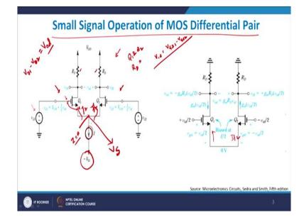
So with this knowledge let me show you how does it work out in terms of working principles. So I can safely say that  $V_{G1}$  is equals to  $V_{G2}$  equals to let us suppose  $V_{CM}$ , right? Let us suppose I have a common mode signal been given whose value is equal to  $V_{CM}$  then I get  $i_{D1}$ equals to  $i_{D2}$  equals to I by 2, right? Because you are drawing i current and then therefore half the current will go to left and half the current will go to right arm.
