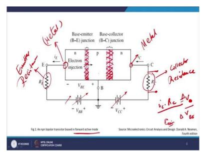
And we define this and we generally therefore put arrow head here and arrow head here assuming means implying that these are variable power sources or variable power supply which is there with you. This  $R_E$  and  $R_C$  are basically the resistances this takes care of the Schottky resistance at the contact because the contact with this side and this side will have metal contact right we had discussed this point earlier also. This will be metal this will be metal also so both are metal.
