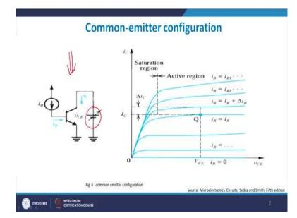
Now if you look very carefully here, when  $V_{CE}$  was equals to 0, right I had 0 current which is expected also the collector current was 0. And if  $V_{CE}$  is equals to 0 the collector to emitter voltage is 0 then I would expect to see 0 current available to me.
