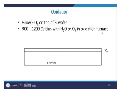
Now, oxidation is you have to grow silicon dioxide on top of silicon and the temperature range is basically 600 to 1200 degree centigrade, right? With  $H_2$  Oand  $O_2$  is basically the reason you are putting this acts as catalyst, right? They act as catalyst means they themselves do not part in the reaction but they hasten the speed of the reaction in a much more detailed manner. So, we use oxidation for doing all these things and it is done at 900 to 1200 degree centigrade.
