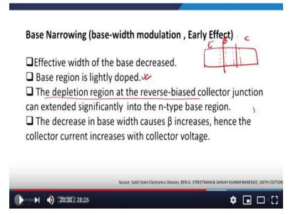
So the depletion thickness at the reverse collector junction can be extended significantly to the n type-base region. We have discussed this point.
