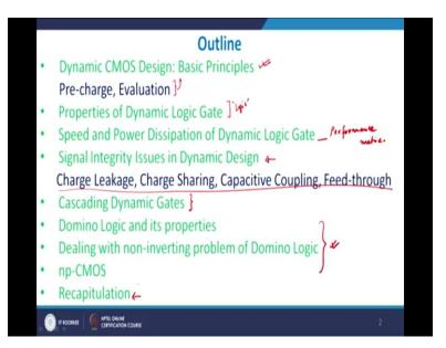
So with this let me come to the first outline of the module and the outlines of the module are: we look into dynamic CMOS circuit design, we understand what is the meaning of pre-charge and evaluation with respect to dynamic CMOS, we look into the properties of dynamic CMOS logic
