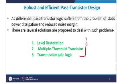
Now as I discussed with you, differential pass transistor logic suffers from the problem of static power dissipation. Why power dissipation? Because now you are directly allowing the output to see the input right and therefore there will be a large current and therefore this will result in a larger power dissipation. So there are certain solutions which is level restoration, multiple threshold and transmission gate. We will take each one of them and explain to you how it works out.
