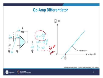
Let me come to the differentiator part, Op-Amp differentiator and if you see differentiator we have just switched to the place of capacitor and register here, so capacitor is here and register is here, so I get i equals to  $C(dV_i/dt)$  differential equation. So, if I take differential signal and
