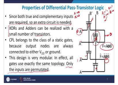
With this knowledge or with this idea, let me come to the next one that let me take up the properties of differential pass transistor logic and let us see how it works out. So since both true and complementary inputs are required, so extra circuitry is needed just to complement the signal. So I require an extra static inverter to complement the signals. Of course, XORs and Adders can be realized using small transistors, one example is given here where XOR and XNOR are designed.
