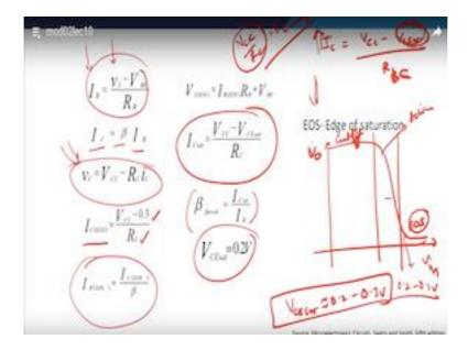
So this is your  $I_B$ , right? So  $I_C$  will be equal to  $\beta$  times  $I_B$ ; a straightforward way of looking at it and therefore, if you multiply this  $I_C$  with  $R_C$  and then  $V_C$  we will be equals to  $V_{CC}$  minus  $I_CR_C$  and I will get from this equation the value of  $V_C$  which is the collector voltage available with me. Therefore as you can remember  $I_{CSAT}$  from here
