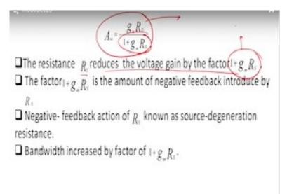
So let me come to this point and this is what I was talking about. So  $A_{v0}$  is equal to minus  $g_m R_D$  upon 1 plus  $g_m R_S$  and therefore, the resistance  $R_S$  reduces a voltage gain by a factor of 1 plus  $g_m R_S$ , this is the reduction. Initially we had  $g_m R_D$  now reduces by factor 1 plus  $g_m R_S$ .
