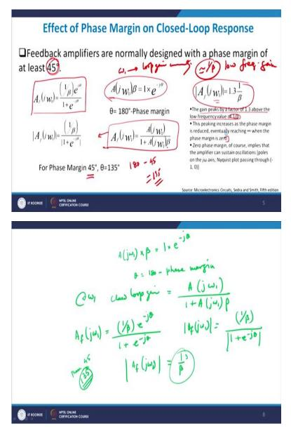
So let us look at the effect of phase margin the close look response, I have the close loop response, close loop means basically I do have feed forward amplifier connected to  $A\beta$  which is basically my feedback network and then it is mixed to a mixture or to a sampler and then the error signals goes again to the amplifier. So this is a basic close loop feedback.
