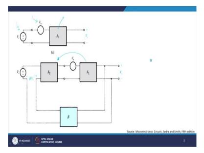
So I am a negative feedback concept here. I have a  $\beta$  here, I have got 2 transistors A<sub>1</sub> and A<sub>2</sub> and therefore you see V0 will be nothing but Vs times A<sub>1</sub> A<sub>2</sub> upon 1 plus A<sub>1</sub> A<sub>2</sub> into  $\beta$ , why? Because now you see your overall gain in the feed forward part will be A<sub>1</sub> into A<sub>2</sub>. So wherever you had A you will be replacing it by A<sub>1</sub> and A<sub>2</sub>, right? So that is what you are doing here.
