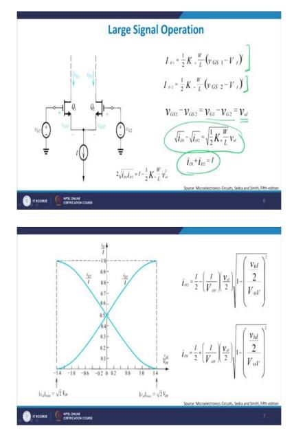
Now with this knowledge which you have gained till now we will do a small not signal analysis here and last signal analysis is required that we have both the transistors here q1 and q2 they are charged with an external voltage source of  $V_{G1}$  and  $V_{G2}$  and there is a current source here which is basically behaving like an ideal current source, which is giving a current I, right.
