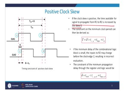
Okay, as I discussed if the clock skew is positive the time available for signal to propagate from  $R_1$  to  $R_2$  and increased by  $\delta$ , I suppose this is clear no need to explain.
