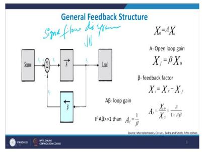
This is referred to as a signal flow diagram. So from signal flow diagram we were able to look at the general feedback structure.
