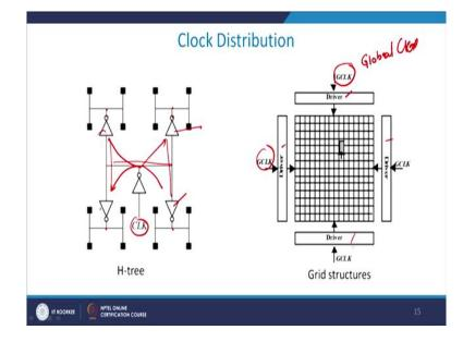
So what I do is, so GCLK is basically my global clock and this global clock actually drives the drivers here which drives the local clock. And this local clock distance is from each of the blocks are so small that you effectively do not get any delay as such.
