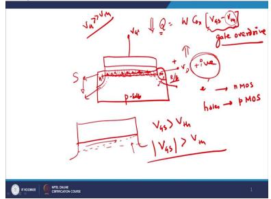
We have also seen that the width, that the total charge which is available is equals to W into  $C_{OX}$  into  $V_{GS}$  - $V_{TH}$  which is, this is known as gate overdrive, right? So higher is the gate overdrive, larger is the charge accumulated which makes sense also because higher the value of  $V_{GS}$ , we have to subtract the threshold because that much amount of minimum voltage will be required to form the channel and excess of that will give you large amount of charge carriers.
