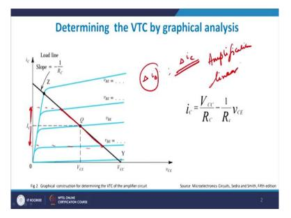
The reason is something like this. The reason is that for equal change in the value of base current, I should get an equal change in the value of a collector current, that is what linearity means. That if I do similar changes in  $I_B$ , I should expect to see a similar change in  $I_C$  also, right? So you see if you change  $I_B$  by this much amount, right?
