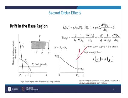
And, all of you can therefore understand that therefore obviously the drift component will have always a component which is primarily proportional to the area as well as to the effective number of charge carriers or number of charge, doping species in that particular point.
