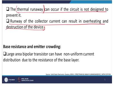
Now, thermal runaway is a standard problem area and if circuit is not designed properly, you will have a thermal runaway which will make the device non-functional and will burn up within a very short period of time. As I discussed with you, runaway of the collector current can be due to overheating and the destruction of the device right. And this is what leads to fatal destruction. Let me come to the third second order effect and that is base resistance, emitter crowding. Now
