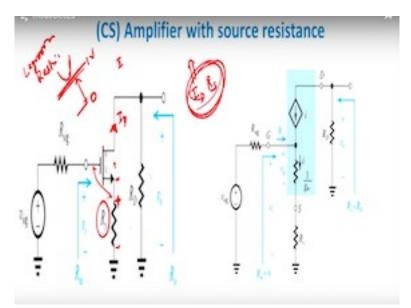
Now let me come to the common source amplifier with source degeneration resistance. So member what change we are doing, what change we are doing is we are replacing the source side which was initially grounded by a source resistance  $R_s$ . So this is source resistance  $R_s$  which is in series to the MOS device, right, so I have a MOS device here and I will put a series resistance here. I have discussed already with you why this is important in terms of application.
