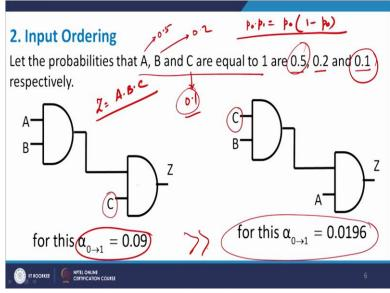
Another methodology which people adopted was what is known as the input reordering. Input reordering means that try to, so let us suppose that the probability of A, B, C equal to 1 are 0.5, 0.2 and 0.1. So A is basically 0.5, B is 0.2 and C is 0.1, the probability that they are equal to 1. Now if this C is inserted, so I have 2 logics. So if you look very carefully, Z is equals to A dot B
