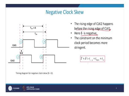
And therefore the rising edge of the clock 2 happens before the rising edge of clock 1 and therefore the  $\delta$  is negative or we define that the clock Skew is negative but the constraint is therefore again as I discussed with you T plus  $\delta$  should be greater than or equal to this. So the positive or the negative Skew does not influence by overall performance. It only tries to make
