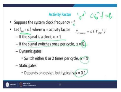
Now suppose a system has system clock of f, then f sw is let us suppose  $\alpha$  into f, but  $\alpha$  is the activity factor. Now if signal is a clock as I discussed with you,  $\alpha$  will be equals to 1 and therefore, I will get CV<sub>DD</sub> square multiplied by f as equals to P dynamic. Similarly, but if the
