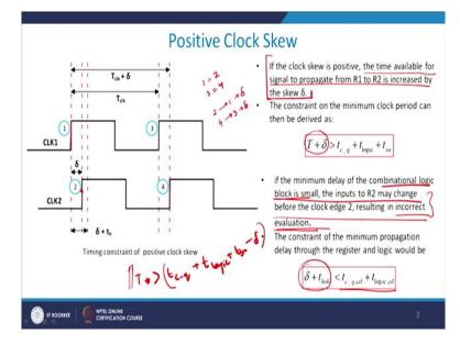
Now if the clock Skew is positive, if the clock Skew is positive which I have shown already then the time available for the signal to propagate from  $R_1$  to  $R_2$  is increased by the Skew factor of  $\delta$ .
