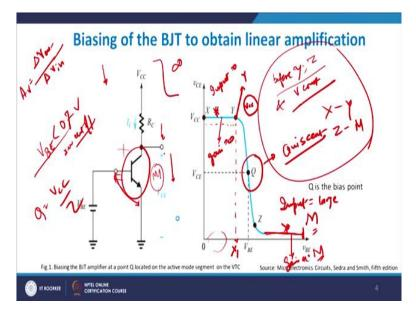
Now if you look at this left hand side figure which is this one, right? I have an NPN transistor which is marked by this red circle let us suppose, right? And what we get is that we bias it by an external source  $V_{BE}$  and we have  $I_c$  and  $V_{CE}$ , right? Now the obvious question how do you physically amplify? When you amplify any signal, how do you do that physically? Well, first of all you apply a DC biased, right?
