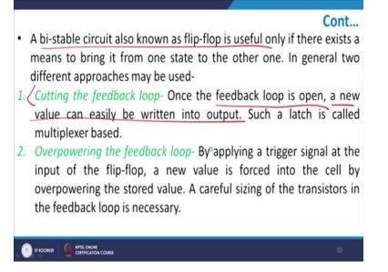
So how do you do it? You when you keep the feedback loop open, no value can be easily written and such a latch is called multiplexer latch, we will discuss this point. We can also overpower the feedback loop by applying a trigger signal at the input of the flip-flop and a new value will be forced on the cell by overpowering the stored value. So if your stored value
