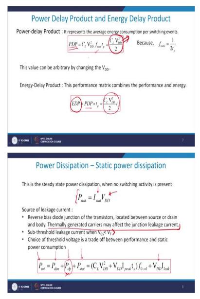
Now, we define a new term which is basically power delay product PDP and it is given by  $C_LV_{DD}$  square by 2 at this stage we need not worry about too much about it and we define energy delay product which is PDP multiplied by tp and therefore  $C_LV_{DD}$  square by 2 into tp gives you the value of your EDP which is energy delay product,
