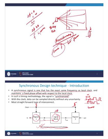
So I have got 2 type of designs one is known as Mesochronous. In a Mesochronous, synchronous we have already discussed. Exactly in phase or equal phase and they are same frequency. Mesochronous have the same frequency, so 2 clocks, so I have a master clock and I have a clock, I have a data train then the data train is said to be Mesochronous provided they have the same frequency but we cannot say it about the phase. So phase will be varying.
