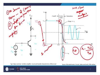
You first insert the DC source, right? You bias the device where, so that it is in the Q-point in the active region for amplification purposes, right? And then superimpose the AC signal, right? Which you want to amplify, right? So you superimpose the AC signal which you want to amplify. So what is the AC signal here?
