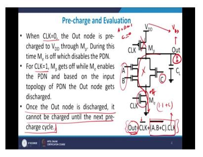
That is what is all written here and so that evaluation, for example, when CLK equals to 0 out will go to, will be pre-charged to  $V_{DD}$ . This will go to  $V_{DD}$ , the out value will go to VDD and this will be disabled or this will be switched off right? A pull down network will therefore be disabled so this will not work and therefore out will go to  $V_{DD}$ , now when CLK goes to 1,  $M_p$  switches off right and based on the values of A B and C out will either go to 0 or remain stable.
