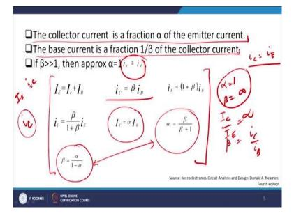
So let me therefore at this stage let me finish off with common emitter configuration understanding. When we meet next time we will start with common base and common collector and that will take care of the effective values here. So what we have learned this lecture is common emitter configuration module and how we can calculate the value of current and basic amplification in a common emitter configuration and we have also learned how I can act as a switch also.
