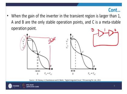
Now if you look at this VTC, then you see this point A and point B are the most stable points, these are the most stable points and the reason being for example, look at the point B, point B is basically Vinput equals to Voutput2 because you feedback directly from the system and this corresponds to  $V_{i2}$  equals to  $V_{O1}$ .
