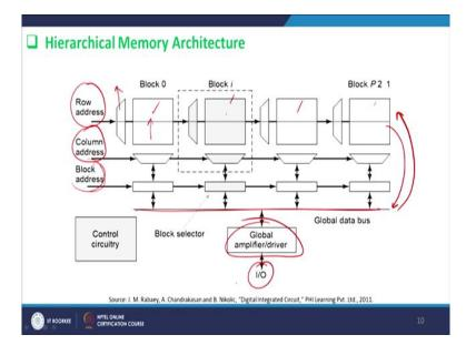
Then we will see that we have Row addresses, we will have column addresses and therefore this row will have Row decoders here and therefore they will be Block 0, Block 1, Block 2, Block 3 so on and so forth and these column addresses will be responsible for taking the column of the block, particular block I will insert the block address here and these will be responsible for talking with these blocks for extracting it.
