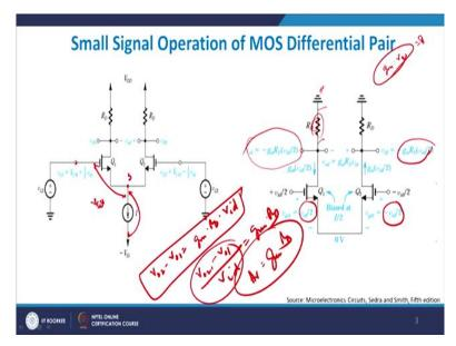
So, let me show to you therefore what is happening here. As you can see a bias state, I have  $V_{GS1}$  equals to  $V_{id}$  by 2 and  $V_{GS2}$  is therefore minus  $V_{id}$  by 2, right? And therefore this much
