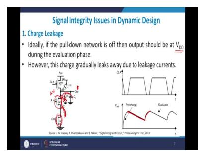
In a dynamic logic, you do have a problem of charge leakage and that is very important or that is very difficult to do that. Ideally, as I discus with you, your pull down methods is off when the output should is at  $V_{DD}$ . So when your output is at  $V_{DD}$  right since your CLK is at low voltage and so this is cut off right? However, there is a problem the problem is that there is a, so when you pre-charge it, your output goes to high value right?
