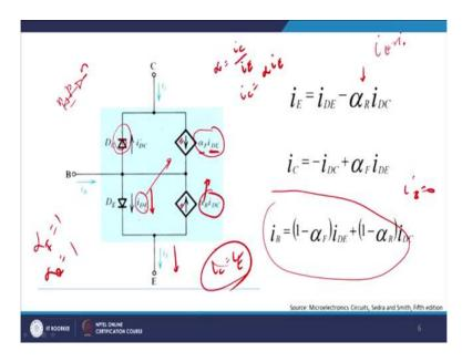
So this is the reason we see  $i_{DE}$  here and base to collector is shown in this manner, because it is an NPN so the diode will be in this direction and it will be in this direction, that is what we are seeing, right. So both P are connected towards base and both N connected toward collector and emitter.
