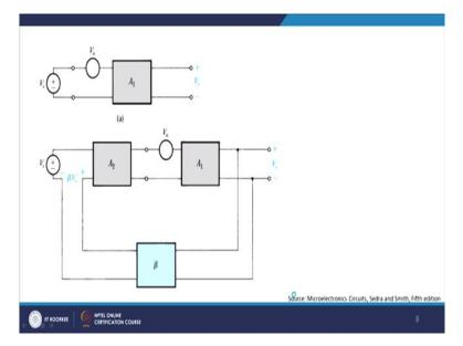
So I have got amplifier  $A_1$  which is basically a noisy amplifier and I have a source signal here and at the input referred noise of this  $A_1$  is basically  $V_n$ . Now what I claim is, that if I had this  $A_1$ , right? It should be preloaded by an amplifier  $A_2$  whose noise source is almost 0, right? If this is the case then I automatically get a much better profile as far as designing is concerned.
