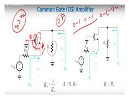
Now, let me come to common gate configuration, in common gate configuration again as I discussed with you the gate will be actually grounded so it is also known as gate grounded configuration, right. So I have a gate grounded configuration what is it means, that my gate is basically grounded which means that the gate is grounded here as you can see and therefore when get is grounded we automatically have a device and if it is an NMOS device it will be basically in a cut-off mode as such.
