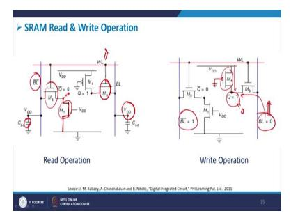
As I have discussed with you the read operation is something like this that you have Q here word line goes high, switches on this  $M_6$  and you are able to transfer this Q onto bit line bar with the one voltage, threshold voltage drop, this appears across this therefore you have a  $V_{DD}$  appearing here. Whereas when you have bit line bar getting activated this goes on,  $M_5$  goes on.
