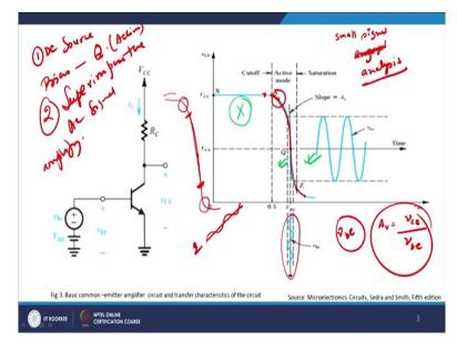
So, I have got if you look carefully I have got this thing that I have got cut-off region which is this one, right? This is the cut-off region then we have the amplification region with the active mode and I have got a saturation region here. So cut-off region, active mode and saturation it will vary depending on the value of  $V_{BE}$  which you are choosing. So depending on the value of  $V_{BE}$  we can think of active and saturation region, right?
