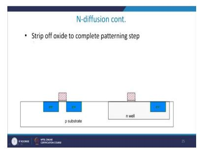
So, next slide as you see I have removed this polysilicon by doing oxide layer. You remove the oxide layer and therefore, what we have done is all the oxide layer here has been removed. If you go back to the previous slide this was the oxide layer which was there. Now, by doing HF etching or using some other technique I can remove this oxide layer directly and I get almost devoid of any oxide layer in this case, right?
