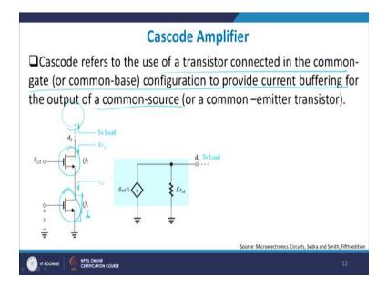
So cascoded amplifier is refers to the transistor in which a common gate is connected to a to a common source. So, common gate is connected to common source. So, you see this 1 is cascoded. This is my common source, right? And q2 is cascoded with respect to q1, right? And if you look very carefully this is so you have a load here and you are driving  $V_{g2}$  and we are giving an input voltage here and you are looking at the output somewhere here at this particular point.
