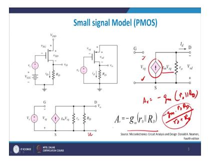
And, this is what we get here, that,  $A_v$  will be minus  $g_m$  times r<sub>0</sub> parallel  $R_D$ , where  $R_D$  is the applied drain resistance which you see.
