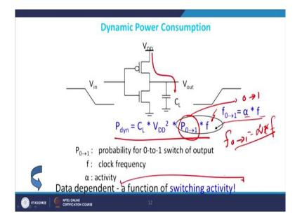
Now let me come to the again the basic dynamics or the basic equations of dynamic power dissipation and if you remember correctly half  $C_L V_{DD}$  square you are taking from the  $V_{DD}$  rail and then you are pushing the half  $C_L V_{DD}$  square into the ground, right. And therefore, for a 1 cycle you are actually taking half plus half which is actually exactly equals to  $C_L V_{DD}$  square and that is the reason you get  $C_L V_{DD}$  square as the dynamic power, initial dynamic power.
