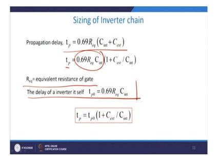
Now therefore sizing up an inverter will reduce its delay because its  $R_s$  getting reduced but this is same instance of time, its input capacitance also increases, so we are not very sure
