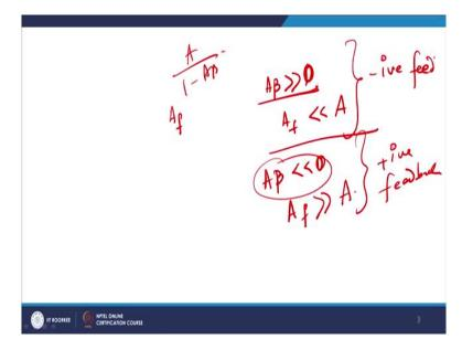
Whereas if A  $\beta$ , so let me write down for you explicitly that if A  $\beta$  is greater than 1 which is in most cases it is then I will get A<sub>f</sub> to be equals to much smaller as compared to A, right? And therefore we refer to this as negative feedback. Whereas if A  $\beta$  is less than 1 then therefore A  $\beta$  is negative and therefore A upon 1 minus A  $\beta$ , A<sub>f</sub> will be always larger than A. As a result this will be actually your positive feedback.
