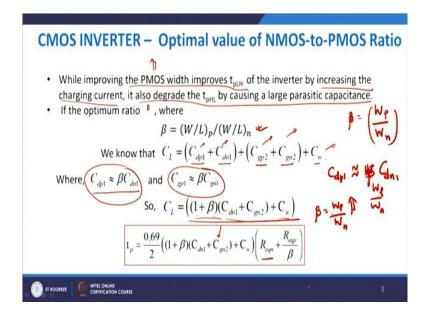
Ok, let me see the optimal value for NMOS to PMOS ratio and now as I discussed with you, while improving the PMOS width right, improving the PMOS width improves  $t_{PLH}$  low to high, if you increase PMOS width  $t_{PLH}$  will go on reducing by increasing the charging current as I discussed with you, but it also degrades  $t_{PHL}$  by causing a large parasitic capacitances,
