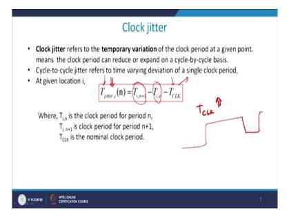
We also discussed clock Jitter that is a temporary variation and we define that to be as  $T_{i, n+1}$  minus  $T_{i, n}$  minus  $T_{clk}$  and so on and so forth that is defined to be as  $T_{Jitter}$ , so if the clock period is very-very high, large then I will get a lower value of  $T_{Jitter}$ . So if my  $T_{clk}$  is large which means that I have a large  $T_{clk}$  I will get a lower Jitter but then you can understand large T means a lower frequency.
