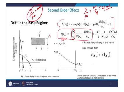
Similarly from Einstein's equation or from otherwise, we can find out that  $E(X_n)$  means electric field at any particular point  $(X_n)$  is given by this formula, the same formula which we get right? And we can from there we can get the value.
