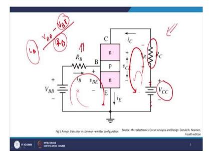
So what we get from here is that yes if  $V_{BB}$  is equals to 0 the base emitter junction will have 0 applied bias right. Why it will have 0 applied bias because with  $V_{BB}$  equals to 0 effectively your base emitter current if I am assuming it to be ideal one is 0. So 0 minus 0 is 0 and I get no current available to us and therefore your base current and the collector current will all be 0.
