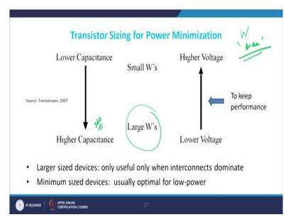
Now, let me come to the transistor sizing concepts, so if you have a small W which means the width is small, I would expect to see, I would expect to see of course the lower capacitance because small W primarily means that the area under the this thing gate is very small and therefore, you require a lower capacitance. Whereas if you make your capacitance higher and higher I obviously at larger W, I get a higher capacitance and therefore, this restricts my 3 dB bandwidth and so on and so forth.
