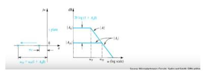
Now, therefore applying a negative feedback as I discussed in your previous turn you are able to increase the bandwidth of the amplifier at the cost of its gain right. Since the pole of the closed-loop of the amplifier never enters the right half of the s plane, you automatically get a dominant much more stable system with you right.
