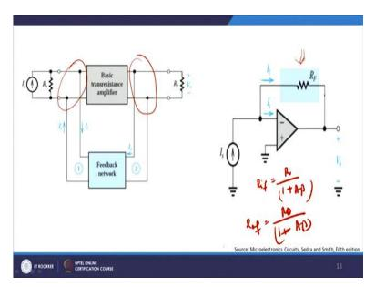
And you see that I am taking a shunt here, I am taking a shunt here and therefore this is my  $R_S$  source resistance, load resistance in the feedback network and one of the best examples is basically your operational amplifier design, wherein you will have  $R_F$  here which is basically,
