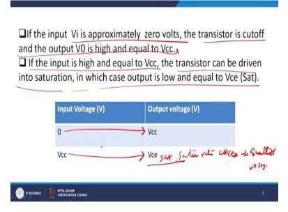
Therefore, as I discussed with you, if the inverter  $V_I$  is approximately 0 Volts input, the transistor is cut off and the output voltage  $V_0$  is high and equals to  $V_{CC}$ . So when you input is low, output is high. Now if the input is high and equal to  $V_{CC}$ , the transistor can be driven to saturation in which case the output is low and equals to  $V_{CEsat}$ . So the output is either equal to  $V_{CC}$  or equal to  $V_{CEsat}$ .
