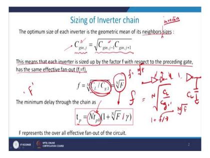
So let me start from there and show to you that therefore, the optimum size of each inverter J<sup>th</sup> inverter is the geometric mean of its neighbouring inverters or neighbouring sizes, right, it should be neighbouring inverters as well, right. So what we are telling you is that J<sup>th</sup> inverter will be basically if you are able to fix its value of input capacitance to be equals to this, then possibly you will get a reduced delay.
