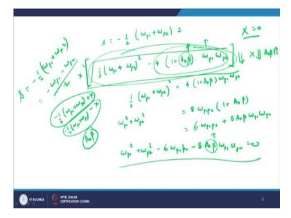
Which effectively means that s will be equal to plus minus. Right? Or sorry s will be equal to minus half  $\omega_{p1}$  plus  $\omega_{p2}$ . Right? And then plus minus taking sign of root over 1 by two  $\omega_{p1}$  plus  $\omega_{p2}$  whole square minus four times 1 plus  $A_0 \beta$  into  $\omega_{p1}$  into  $\omega_{p2}$ . So this are the two roots of the equations, one root is with the positive sign another root will be with respect to the negative sign.
