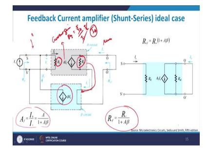
Now, let me come to the case of feedback sorry feedback resistances over here, feedback shunt resistance feedback shunt series resistance. So, I get a shunt series basically means that I will take a parallel output here. And I will do a series input at this particular point, right? And therefore, you see I have got  $R_i$  here and then  $A^*I_i$ . A is basically my current gain, right? And is given by  $A_i$  and this will be current gain which is which is visible to me.
