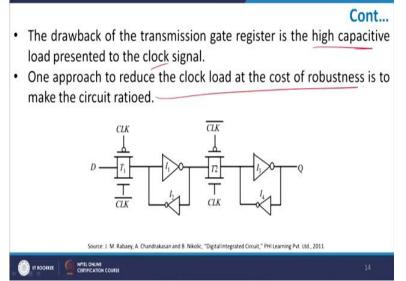
The drawback of, as I discussed with you is the high capacitive load and robustness of the circuit is an important issue.
