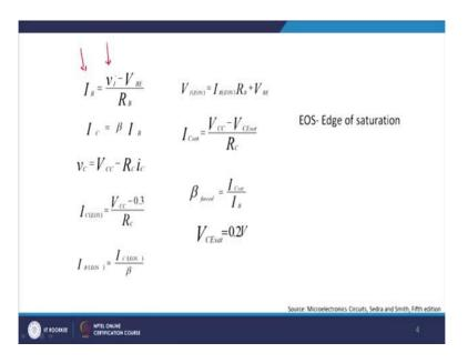
So if you look at this figure or in this equation you can see that the  $I_B$ , the base current can be given as  $V_I$ ,  $V_I$  is the input voltage minus  $V_{BE}$ , minus  $V_{BE}$  why?
