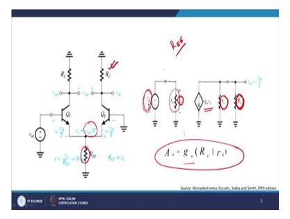
The advantages it is much easier to calculate various formulas from differential half circuits. With this knowledge, let me therefore come to a small signal characteristic of the differential amplifiers. As you can see my input voltage, I have already told you is differential  $V_d / 2$ , right so I have giving  $V_d / 2$ , this r <sub>pi</sub> is nothing but the input side resistance offered by the differential pair. So, it is basically the pairs r<sub>pi</sub>, right.
