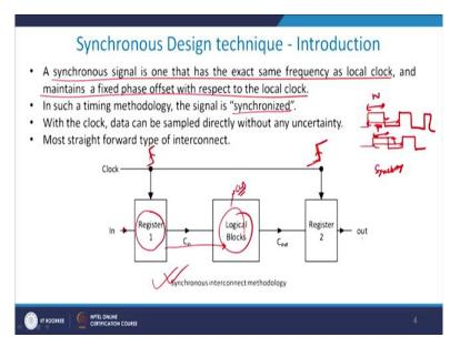
Now let me therefore define certain definitions I will explain to you. Asynchronous signal is one that has exactly the same frequency as the local clock and maintains a fixed phase offset with respect to the local clock. Which means that if I have a local clock which is coming like this, this is a local clock than if I were clock which is something like this, so this is T, this is also T.
