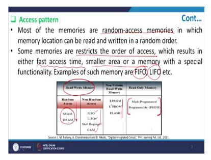
Now how do you access the memory and that the most important part as far as timing and frequencies are concerned. Most of the memories which you will study is the random access memory means which is basically that I can read or write any cell in a random order.
