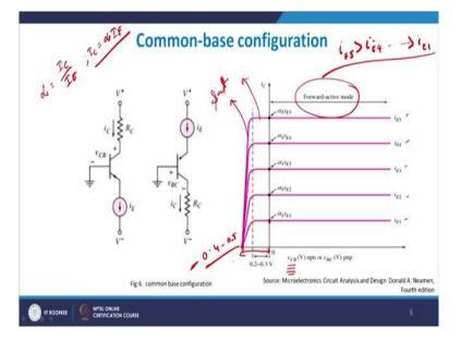
So I have a biased positive so when it is 0 bias even when it is 0 biased. You will see that you still have large amount of current flowing through the device. And the reason being very simple that even at 0 bias you have applied such a large electric filed because of the  $V_{BB}$  that electrons which were predominantly my emitter current  $I_E$ , right passed through the base region very fast and they cross through this region very fast and reach the collector side.
