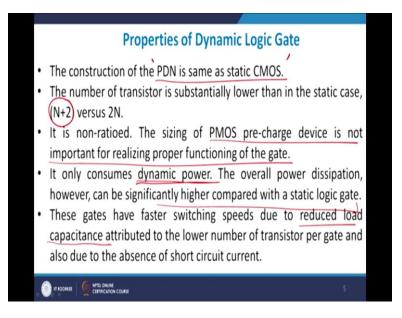
What is the property of dynamic logic? The construction of PDN is therefore exactly the same as a, the construction of the PDN is the same as your static CMOS logic. We have already done that. So PDN network is exactly the same. However, it is much lower than static the CMOS logic. You actually require N plus 2. N plus 2 why? Because N is the number of pull-down networks and plus 2 because 1 pre-charge transistor and 1 evaluation transistor. Of course, it is a
