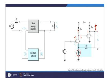
From this physically, let me explain to you how I get negative feedback, so as I discussed with you as this VS increases, this voltage increases, this current increases, so your this voltage drops down, which means that this current here will drop down, which means that this voltage will increase, so with increase in  $V_s$  here I get an increase in voltage here right, but this increase in voltage is primarily means that my  $V_f$  we also go on increasing.
