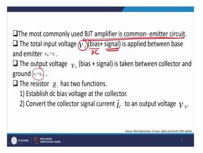
So with this we have understood the basic amplification process of a BJT, so as I discussed with you earlier also, in the earlier module as well as in this module the most commonly used BJT amplifier is the common emitter amplifier, right? So common emitter amplifier or common emitter circuit is the most commonly used amplifier design. Now, my input signal as I discussed with you, will always be a sum of the DC bias plus the signal which you applied, right?
