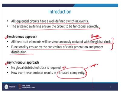
So that is one important clock that there will be a global clock. And therefore the functionality will ensure that by the constraints of clock generation and proper distribution. As I discussed with you therefore that clock going into the system and generating an output logic will depend therefore on the proper synchronization of the clock with respect to individual blocks of the sequential data. This is for the synchronous approach.
