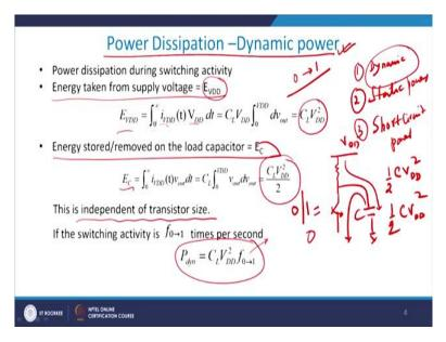
Typically a transistor or an inverter will have three types of power, one is known as dynamic power, right, the other is known as basically a static power, this is static power and third one is actually referred to as a short circuit power, we will explain each one of them individually, but let us first understand dynamic power, right.
