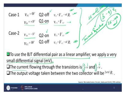
With this knowledge or with this basic idea, let me therefore move on. So, as I discussed with you in the first case Q 2 will be off and therefore V C1 will be equals to  $V_{CC}$  minus alpha I times R<sub>C</sub> and  $V_{B1}$  when it is plus 1 volt Q 1 will be on and then V<sub>C2</sub> will be equals to  $V_{CC}$ . So, whichever the transistor is off the output will be latched to  $V_{CC}$  and whichever transistor is on the output will be latched to  $V_{CC}$  minus alpha R<sub>C</sub>.
