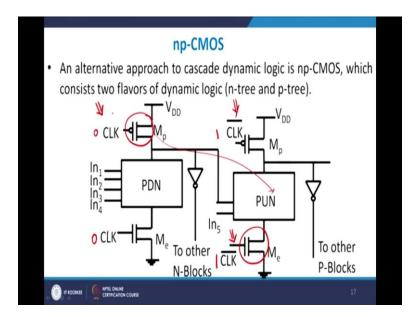
And that is the problem area for this logic taken into consideration. Another alternative approach is using NP logic. NP logic what we do is that, it is exactly the same as domino logic only thing is that we have a do is that we have a dynamic logic with CLK and CLK and then we drive it with a dynamic logic with CLK bar. So whenever your CLK is high so when CLK is suppose high or suppose CLK is low so this is low, this is low but then this is high and this is high.
