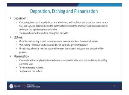
Let me come to deposition. When deposition is conducting layers such as poly-silicon and aluminium, and insulation and protection layers such as silicon dioxide and silicon nitride and they are done by CVD process at high temperature high temperature chambers. So, I have a high temperature chamber, right? So, once I do a CVD which is a chemical deposition and I deposit layers of silicon dioxide and nitride which is both by the way directive in nature over this area.
