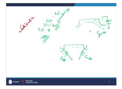
This is the basic model of a MOS capacitor. The third or the fourth type of junction capacitance which you feel is basically, please remember as I was discussing with you just now that your source and drain region, right remember is always sort of a reversed biased at least the drain region is reversed bias which means that there will be always a depletion capacitance at this particular point, right.
