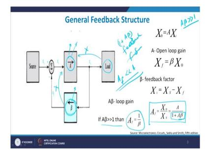
It means that, you have this load, right? We have this load, so this might be resistive load. Now I am assuming that resistive loading or for that matter this  $\beta$  does not load my amplifier in this manner or this does not load in this manner. There is no loading effect, right? So there is no loading, so I am assuming that. Then, second assumption is that my signal through my feedforward is always moving from input to output, so there is no reflection of signal within the amplifier itself.
