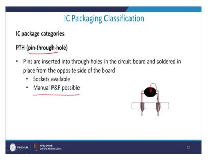
IC packaging, well there are 2-3 important packaging techniques, the first is a pin-throughhole. Pins are inserted through holes as you can see here in the circuit board and soldered in the place in the opposite side of the board. So this is soldered from where? So this is through holes and then you soldered it here right, so manual PNP is possible manual pin through holes can be possible and you can actually solder it manually to a larger extent.
