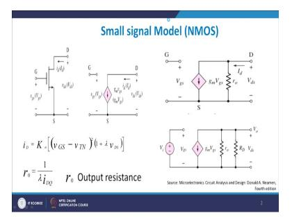
With this knowledge, let me come to, very important topic that is known as a small signal model of a device. So, we have understood NMOS, NMOSFET and let us, therefore, take the NMOSFET and see, if we can do small signal model, means by the input voltage is varying by very small.
