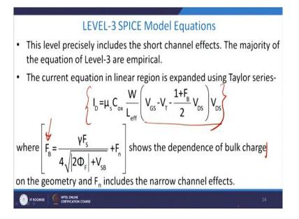
And it is given by this formula here,  $I_D$  equals to  $\mu_S$ Coxide, W by L, this  $F_B$  is basically my geometry dependent idea and that varies with the level which is there. Most of the time we do not use level 3, most of the time for our practical purposes level I and level II is the most seldom used SPICE model file for our practical applications.
