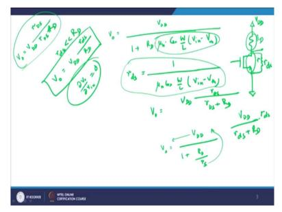
So we can write down therefore with this explanation, we can write down V<sub>0</sub> to be equals to  $V_{DD}$ ,  $V_{DD}$  divided by 1 plus  $R_D$  times  $\mu_n$  times C oxide into W by L into V in minus V TH and you get this. The effect was  $R_{DS}$  as the drain to source resistance as 1 by  $\mu_n$  C oxide W by L V in - V TH and therefore I can write down V 0 to be equals to V<sub>DD</sub> into  $R_{DS}$  into  $R_{DS}$  plus  $V_{DS}$  R<sub>D</sub>.
