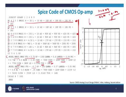
So, let me come back to this point basically if you look at graph here this is V out versus V in which is basically also referred to as VTC, so this is basically the VTC often operational amplifier. So you give an input swing from minus 0.2 to plus 0.2, right?
