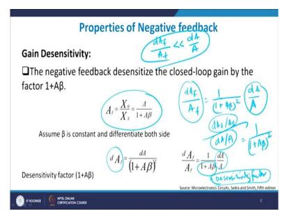
With this general property let me come to the properties of negative feedback. The first property of negative feedback is, the gain is desensitized which means that though our gain reduces in case of negative feedback, but the gain itself is desensitized which means that the gain is now more stable independent of frequency, independent of any of the systems available to us, any of the device parameters or circuit parameters independent of that.
