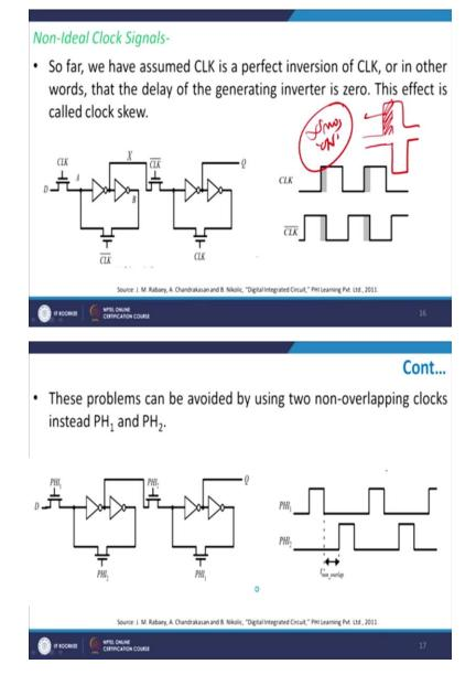
So as I discussed with you non-ideal signal will be those signals which the clock is a nonperfecting clock and this can be done by using two overlapping clocks of just pure nonoverlap of each other and we should be able to generate the output file.
