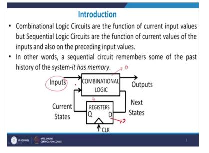
See, if you look here in this slide, you will see that this register has to be minimum delay. Suppose this register would have 0 delay, then what will happen? That, you send an input at this point, at this point you send an input and exactly that say, assuming that this has got 0 as the delay, this has also got 0 as delay, that instantaneously as you insert input here, you will get an output at this particular point.
