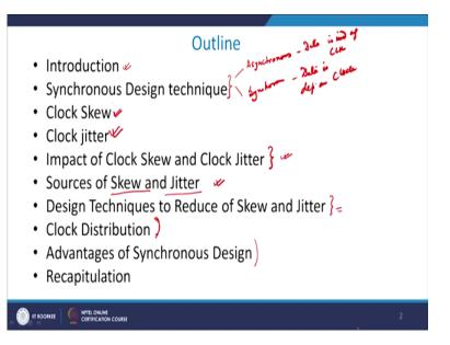
We will first introduce to you the basic concept of timing and then we will look into the synchronous design techniques. As they have discussed earlier there are 2 types of design, one is A synchronous, right? And we have another is synchronous. What is A synchronous? Well, Asynchronous is that when the data is independent of clock, right? External clock and when data is dependent on clock we define that to be as Asynchronous design.
