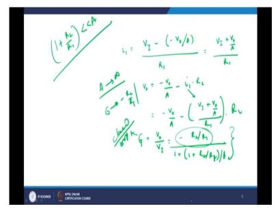
So I get current  $i_1$  equals to  $V_I$  right minus minus  $V_0$  by A. Why  $V_0$  by A? By  $R_1$ .  $V_0$  by A is output voltage by A will give you the difference in the input voltage. So,  $V_I$  minus that by  $R_1$  is the current. So, I get  $V_I$  plus  $V_0$  by A by  $R_1$  equals to  $i_1$ . This  $i_1$  flows through  $R_2$ ,  $R_1$  and  $R_2$ , the same current is flowing. So I get  $V_0$  equals to minus  $V_0$  by A minus  $i_1$  into  $R_2$ , right.
