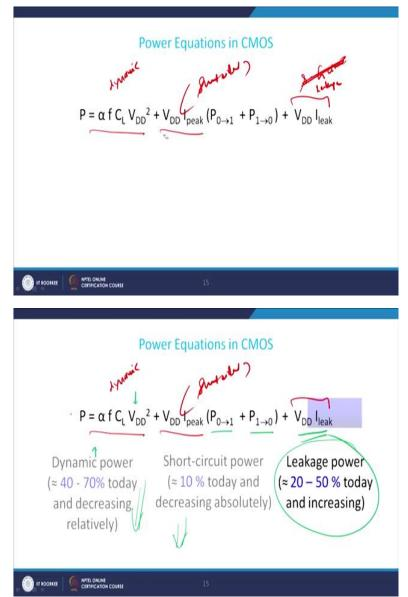
Next we get the power equation, the power equation as I discussed with you  $C_L$  f times  $V_{DD}$  square is your dynamic power dissipation, we have  $V_{DD}$  times I peak as the so this is basically your, so this is a dynamic, this is your short-circuit, short-circuit power dissipation, this is your not short circuit, this is a short circuit, short circuit, circuit power dissipation and this is basically your power dissipation by virtue of leaking so I have a leakage available with me.
