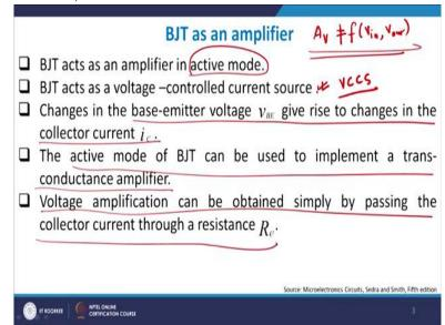
Now therefore so that is what I was saying that, so the last point is that a voltage amplification, right can be obtained simply by passing the collector current through a series resistor ( $R_c$ ). So you have  $i_c$  available with you because of a collector current is available with you. Now if the collector current you are forcing it to pass it through a resistance  $R_c$  then  $i_c R_c$  is basically the drop of the output voltage, right?
