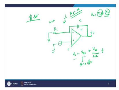
Let us see what happens otherwise, what is the problem otherwise, let me say that you do have a problem that there is a off-set voltage, which means that, so what is the meaning that, it primarily means that if the differential voltage Vid between the 2 terminals of op-amp is zero the output should be exactly equals to zero. Because, A into  $V_{id}$  is equals to output is equals to  $V_{out}$ . Ofcourse the common mode signal is there but this is the output voltage.
