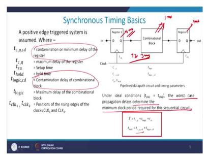
So  $t_{hold}$  is equals to  $t_{c-q,cd}$ , what is  $t_{c-q,cd}$ ? It is the contamination delay of the register of the minimum delay of the register plus  $t_{logic,cd}$  which is contamination delay or the minimum combination and you can understand why? So this logic will have say one millisecond delay, right? And then this is having 1 millisecond delay, right? And let us also assume that this is having 1 millisecond delay.
