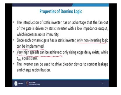
Since each dynamic gate has a static inverter only non-inverting logic can be implemented but obvious very high speeds can be achieved in this case and the reason being that  $t_{PHL}$  being approximately equals to 0. High to low will be approximately equals to 0 right? Now the inverter can be used to drive bleeder device to combat leakage and trans distribution.
