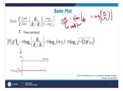
Now, let me come to a very important term or a very important aspect of designing is basically the Bode Plot. The Bode Plot is basically this one, the variations of the (gain) voltage gain in dB with respect to frequency in log scale because, if you remember frequency can vary from 0 to maybe gigahertz value or maybe megahertz or gigahertz value.
