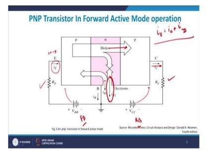
The same concept as in the previous case the only thing is the polarity of the battery will now be changed or reversed and you will have  $V_{BB}$  in which the positive end is connected to P type and  $V_{CC}$  the negative end is connected to P type. So this will be reversed bias and this will be forward biased so we are keeping the same concept exactly the same as in the previous case and trying to formulate a policy for finding out the current.
