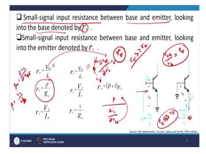
And now we define another resistance known as the small signal input resistance and it is referred to as  $r_{\pi}$ , right? And it is nothing but the resistance looking from the base side where between base and emitter, right? So looking from the base side, if you're looking from the base side the resistance offered by this is basically  $V_{be}$  by  $i_B$ . So  $V_{be}$  is the voltage which you see between these two points and  $i_B$  is the current by virtue of this voltage.
