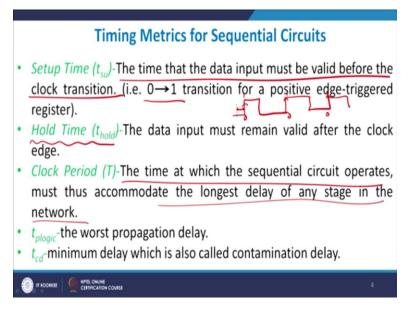
Of course, the time at which the sequential circuit operates must thus accommodate the longest delay of any stage in the network. I hope you can understand this point, from the previous diagram you understand.
