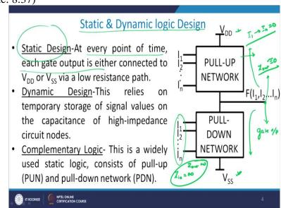
Now static logic primarily means that at every point of time, each of the gate output which is this one, this is the gate output, right is either connected to  $V_{DD}$  or  $V_{SS}$  via a low resistance path.
