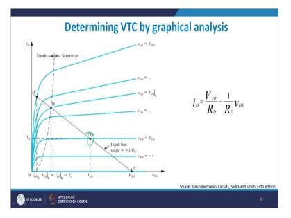
But I wanted to stress again here one important point is that just as you saw in the previous case, try to keep your Q point in the middle of the saturation region rather than in the edge here at the edge here that makes sense also. So we have understood the saturation region and we have understood the voltage gain
