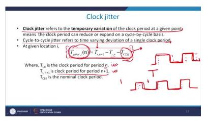
And as you can see therefore there is a cycle to cycle refers to time varying deviation of a single clock period. So you had a single clock period of capital T. Now because of cycle to cycle variation in the jitter your new value at location I will be given as  $T_{i \text{ jitter}}$  to be equals to  $T_{i(n+1)}$  minus  $T_{in}$  minus  $T_{clk}$ , where  $T_{in}$  is basically the clock period for period n and  $T_{in}$  plus 1 is for n<sup>th</sup> plus 1.
