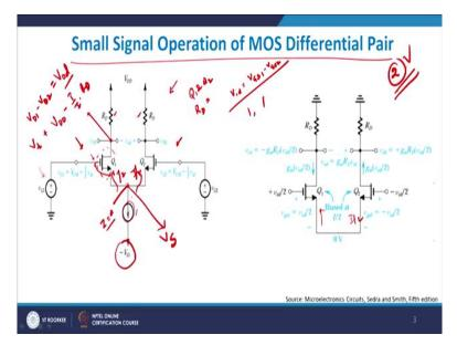
If you look very carefully here is the voltage at this particular point, this is  $V_{DD}$  minus I by 2 into  $R_D$  is the voltage at this particular point. You are added  $V_t$  to it threshold voltage of this device Q1 this has to be the minimum voltage. See, if my voltage falls below this, right? Say my threshold voltage is, my  $V_t$  is say 1 volt and  $V_{DD}$  minus 1 by 2  $R_D$  is equals to say 1 volt again.
