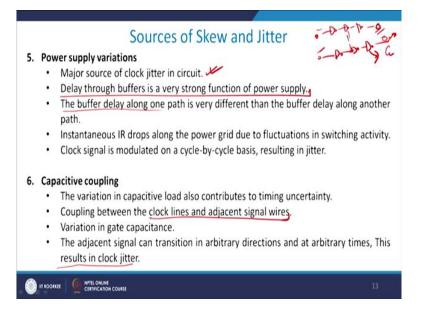
Similarly the delay through buffer is a strong function of power supply we have studied this when we were discussing FO4. Similarly the buffer delay between any 2 path, so I would delay here and I am putting buffers here.
