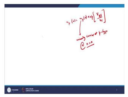
Now what does it tell me about this thing. So if it is  $n_PX$  equals to X is the distance from the base region  $n_P0$  exponential  $V_{BE}$  minus by  $V_T$  as you can see from this concept or this basic idea  $n_P$  means n suffix p means this is basically minority carriers minority carrier concentration, carrier concentration at P type base at X equals to 0.
