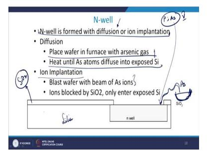
We come to the n-well formation. Now, n-well basically meaning that you are doping with either n type dopant concentration which is basically either phosphorus or arsenic, right. This is group V element which you are doping with and what you do is that this n well is formed with diffusion or ion implantation, right? So, typically in most of the organisation or fabrication techniques we use diffusion, right?
