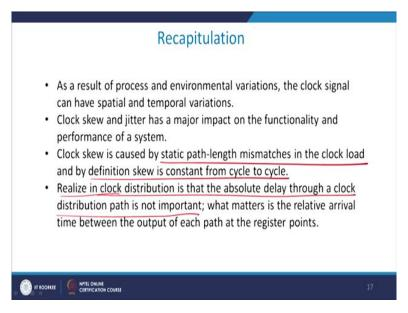
So let me recapitulate the whole lecture which we did for the 2 parts of clocking sequences. We saw that what is the clock Skew, we also saw what is the clock Jitter, they effect the functionality and performance of a system. Clock Skew as I discussed with you is caused by the static path-length mismatched in the clock load and by definition clock Skew is constant from cycle to cycle.
