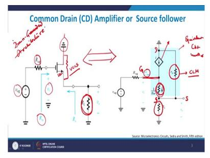
So, if you come back here, you are looking from the Drain side onto the device, means you are looking from this side onto this side which is nothing but 1 by  $g_m$  as we discussed earlier.
