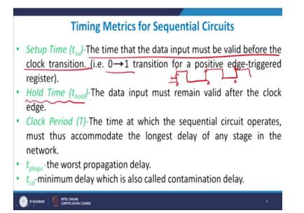
Let me come to the second definition which is known as hold time. Hold time is again very simple, the data input must remain in the same state after the pulse has passed, so setup time is before the pulse has come, arrived and hold time is after the pulse has arrived, you should actually require to have this much.
