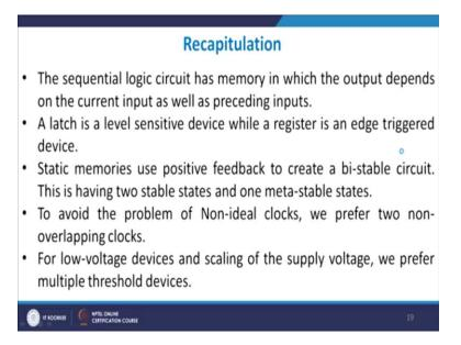
So let me recapitulate what we have done in this small module, we looked into sequential logic design, how it's made, what are the diagrams we have already seen it. A latch is a level
