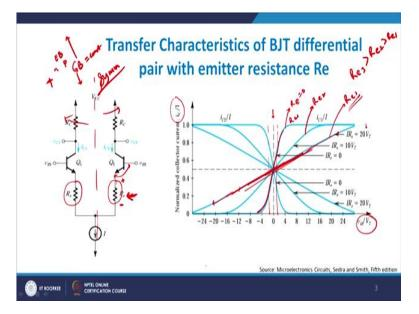
How do you do it? Well the methodology which people adopted was that they inserted a resistance  $R_e$  in series to the (emitted region) emitter region and if you plot there for the graph between  $i_c$  by I which is basically collector current normalize with respect to total current versus  $V_{id}$  by  $V_T$ , the same graph as the above, you see as the  $R_i$  value becomes larger, right.
