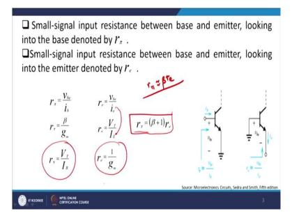
Similarly  $r_e$  therefore can be written as  $i_e$  is the emitter current and  $V_T$  is the base to emitter voltage at 300 mV we will write it as  $V_T$  thermal equivalent voltage. Therefore I can write down that  $r_{\pi}$  could be written as  $\beta$  plus 1  $r_e$ , right? And you can do it yourself to find out this value that means  $r_{\pi}$  is approximately  $\beta$  times larger as compared to  $r_e$ , right?
