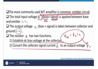
The resistor  $R_c$  has two functions. We have already discussed this point  $R_c$  will help you to establish a DC bias, so higher is the value of  $R_c$  slope will be lower but with a negative sign, right? And lower the value of  $R_c$  higher will be the slope with a negative sign. The slope is from the side, it is not like this, it is like this. So you will always understand that the slope is negative in the sense.
