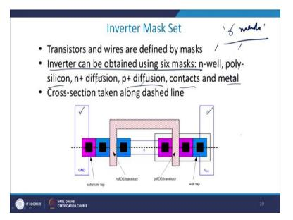
Now, let me come to the inverter mask set, right? We have got transistors and wires are defined by masks. So, these are basically the masks which are available with you. And inverter can be obtained by using 6 masks; n well, poly silicon, N + P + diffusion contact and metal, contact and metal. So, it is 1, 2, 3, 4, 5 and 6. So, you require 6 masks in order to do it right and 6 masks can easily be purchased and can be used.
