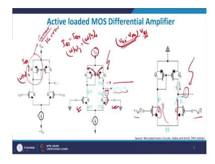
This action is basically known as current mirroring, this, this is known as current mirroring, because this, I will explain it to you later on maybe current mirror. The reason being that the current flowing through Q3 will be exact if the W by L ratios of Q3 and Q4 are same the current flowing through Q3, suppose this is  $I_{Q3}$  will be exactly equals to  $I_{Q4}$  provided W by L of Q3 is exactly equals to W by L of Q3 is exactly equals to W by L of Q4.
