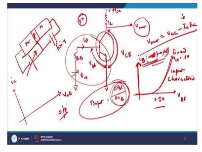
Quite interestingly let me also show to you if I want to plot  $I_B$  versus  $V_{BE}$  versus  $I_B$ , this is also known as input characteristics. So base current  $I_B$  versus  $V_{BE}$ , right for a fixed value of  $V_{CE}$ , right. So my  $V_{CE}$  is fixed  $V_{CE}$  I vary  $V_{BE}$  and try to take the value of  $I_B$ , right. So if you look very carefully for a fixed value of  $V_{CE}$  this starts so this starts to behave like a PN junction diode so in a forward bias condition.
