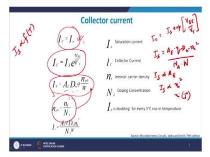
Now as you can see here  $I_s$  is given by this formula because I just replaced  $I_s$  by  $A_E$ ,  $D_nq$   $n_p0$  by W, again assuming 0 charge carriers on the collector base
