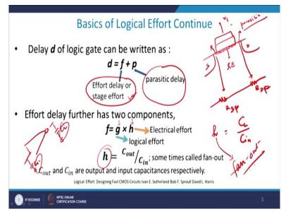
Now, the delay of a logical gate d can be therefore, broken up into two parts, one is known as a stage effort or effort delay and another is the parasitic delay, what is a parasitic delay? Well parasitic delay is very simple straightforward we already discussed this point earlier also just to refresh your memories, I will just do it, let us suppose you have a gate here and you have a gate here and you have a source and drain here, right?
