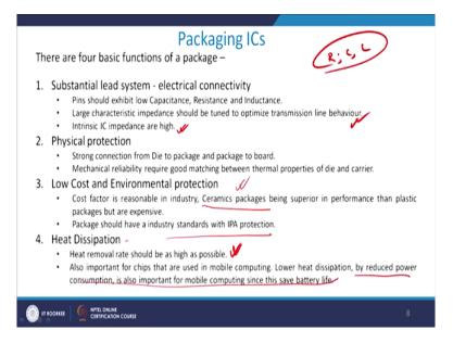
Let us look at the packaging of IC, well there are 4 basic functions of the package. Generally, you should have pins which will be IO pins means input output pins, they should exhibit low resistances, capacitances and inductances so that the delays are minimise across the pin. It should also have large characteristics impedance to reduce the noise at those particular pins which is the second part. And intrinsic IC impedance should be high which we have already discussed in the second part.
