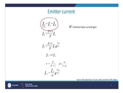
So this is basically a charge conservation principle, the charges is always conserved irrespective of the type of device you take irrespective of the material of the device you take. So  $I_E$  is equal to  $I_C + I_B$  because you will be following the Kirchhoff's law and since you will be following the Kirchhoff's law the total emitter current which is entering into the system must be exactly equal to the total.
